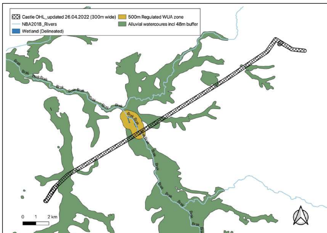
Figure 6-33: The confirmed watercourses and wetlands within the study area, inclusive of the respective buffers and the 500m Section 21c&i regulated water use zone.
