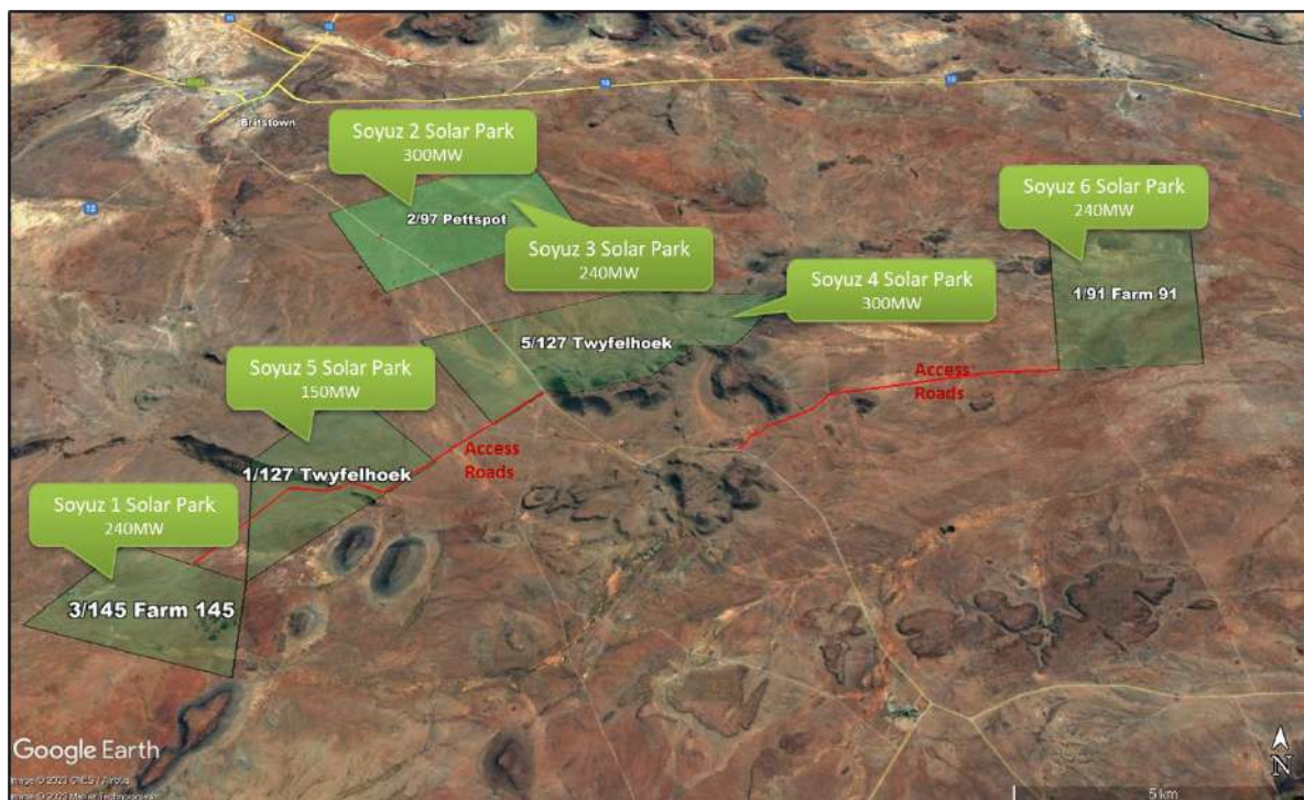
Figure 2 Soyuz Solar PV Cluster 1-6 Overall Layout
