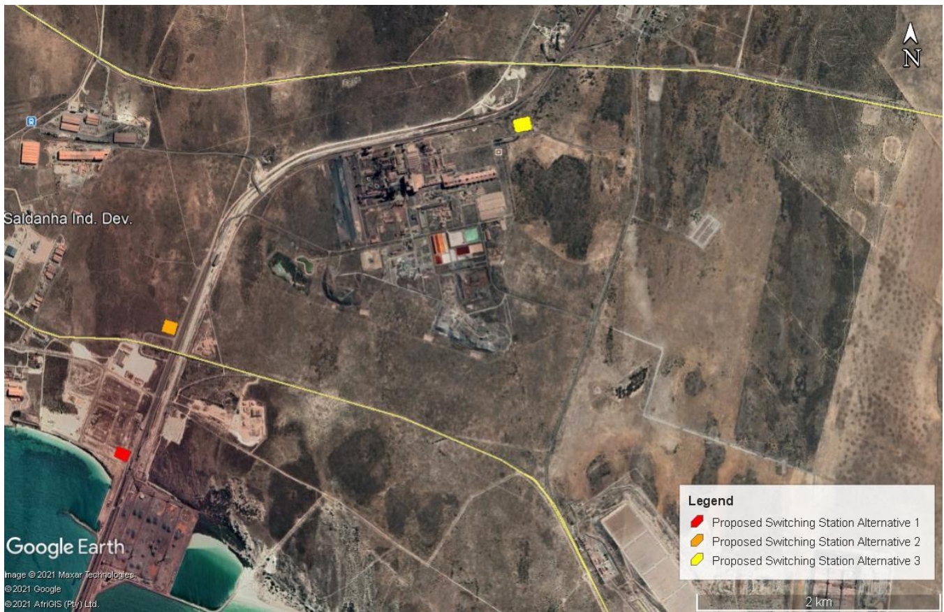
Figure 7-3: Deviation – New Switching Station
