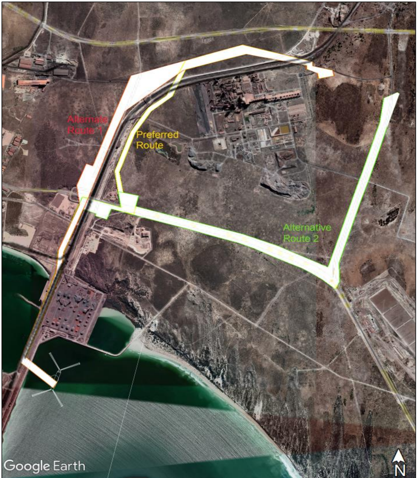
Figure 2-2: Overall Project Layout showing alternative corridors (Transmission).
