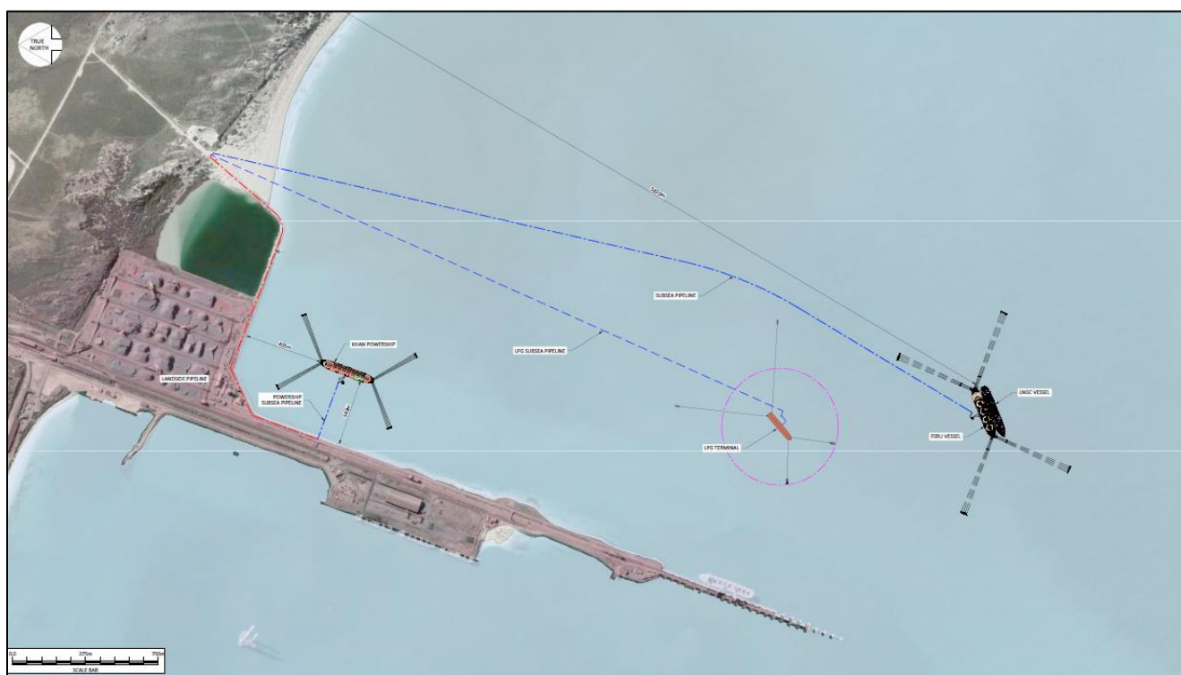
Figure 2-4: Image showing the proposed gas pipeline route from the FSRU to the Powership position in Big Bay.
