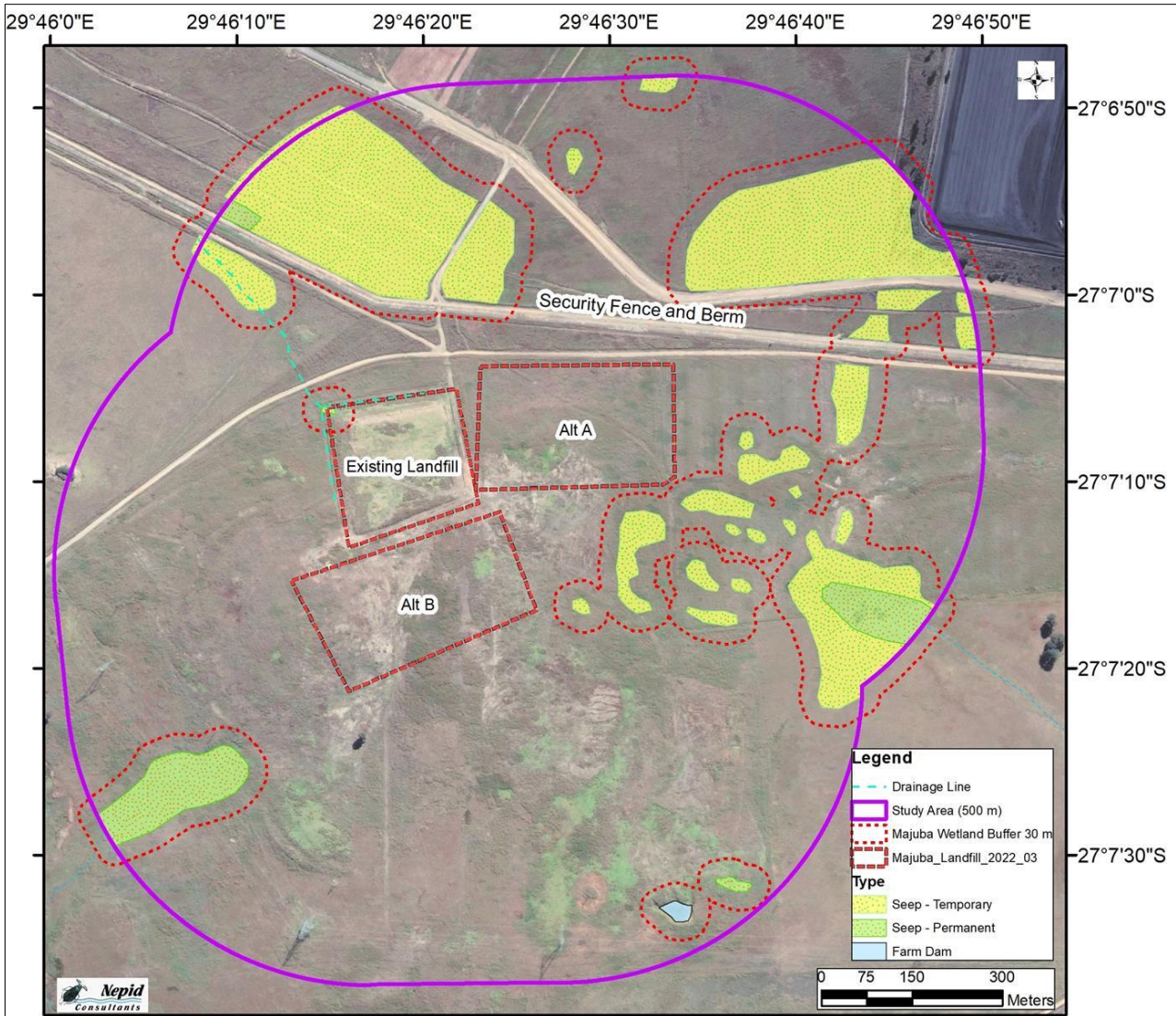
Figure 5.16: Delineated wetlands in relation to the development footprint alternatives, with buffers and the 500m regulated WULA zone (arrows indicate direction of surface flow)
