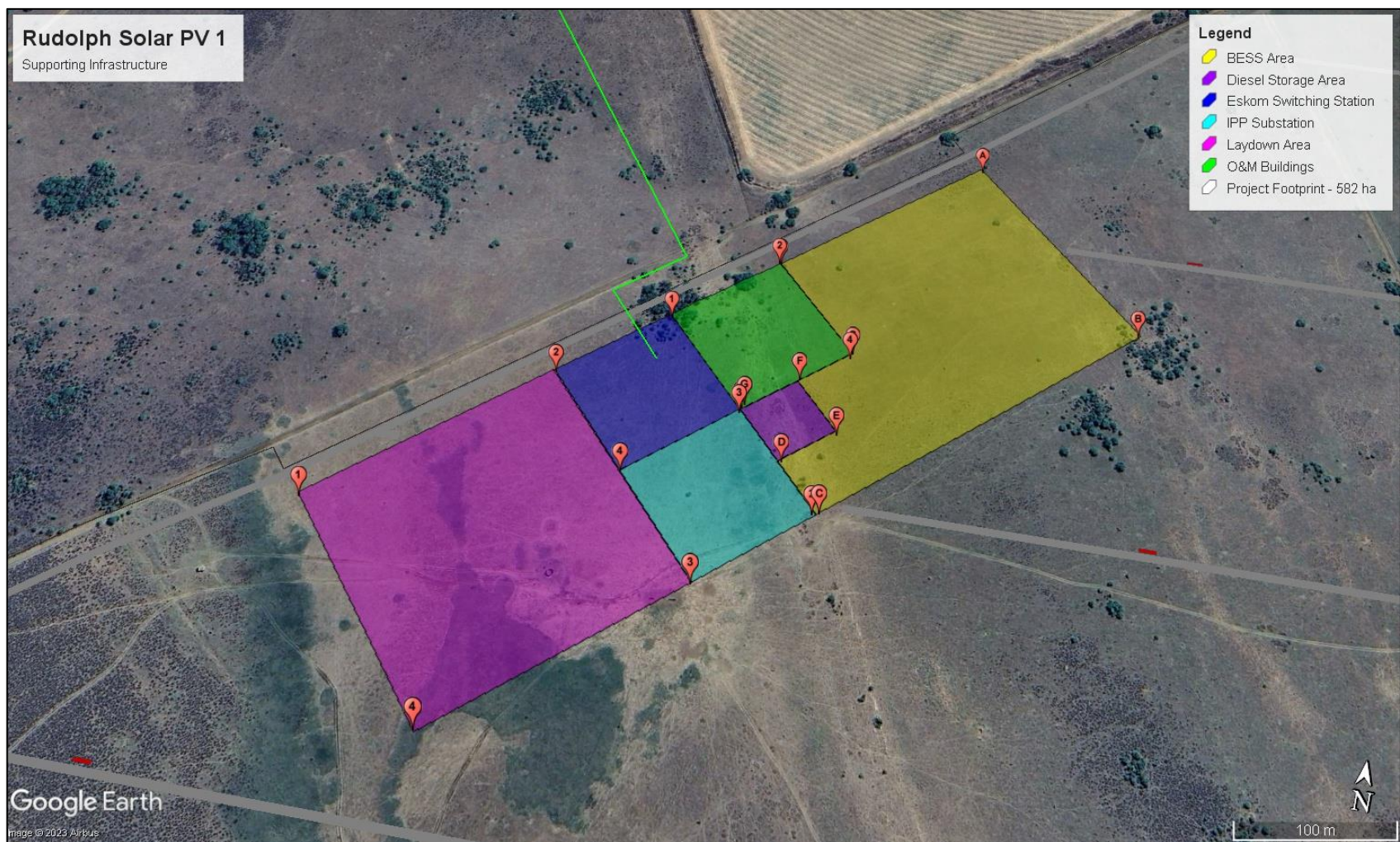
Figure 2.2: Co-ordinate points of supporting infrastructure
