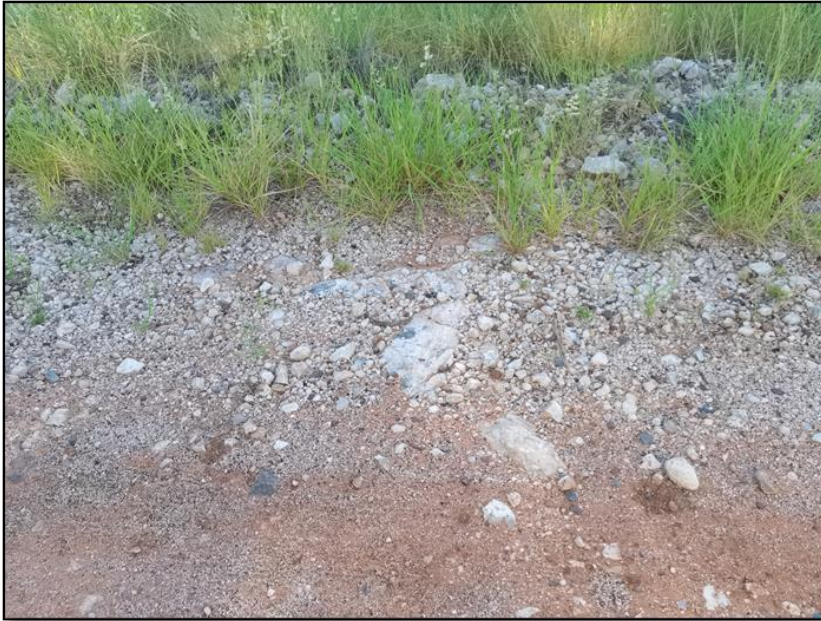
Figure 6.7: Coega soils within the study area where hard carbonate chunks can be seen on the surface
