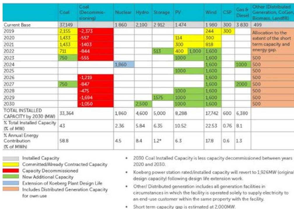
Figure 4.3: A snapshot of the updated Energy Mix as per the IRP 2019
