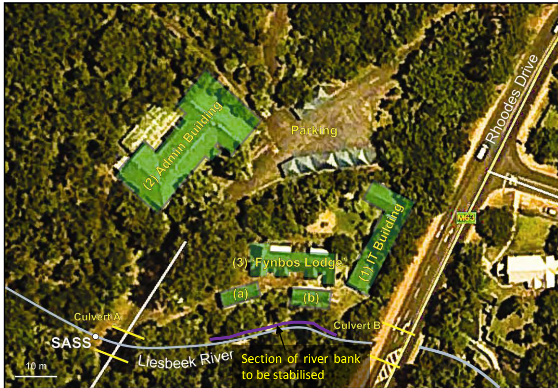
Figure 2 Site Plan showing the existing parking lot, together with: (1) the existing IT building, (2) the administration building and (3) the 'Fynbos Lodge'. The Liesbeek River flows to the south of the proposed development through two culverts between the entrance road to the administration buildings (Culvert A) and beneath Rhodes Drive (Culvert B). The white dot indicates where SASS aquatic invertebrate samples were collected.
