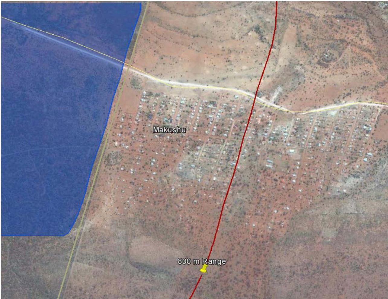
Figure 16: 800 m range influence from maximum charge
