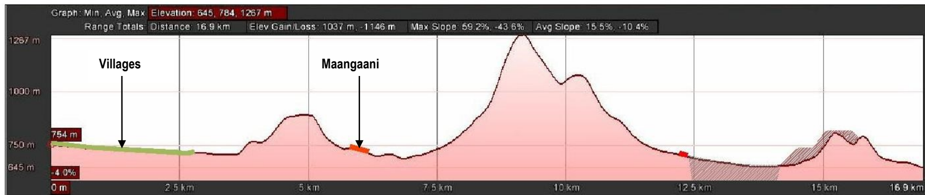
Figure 15: Cross Section D conceptually illustrating the proposed plant (indicated in red) and the proposed waste dump and open cast pit (hatched areas) and in relation to surrounding topography and potential receptor sites.
