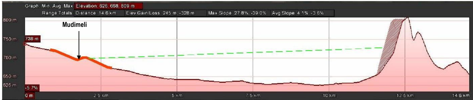
Figure 16: Cross section E conceptually illustrating the proposed waste dump (hatched area) in relation to surrounding topography and potential receptor sites.
