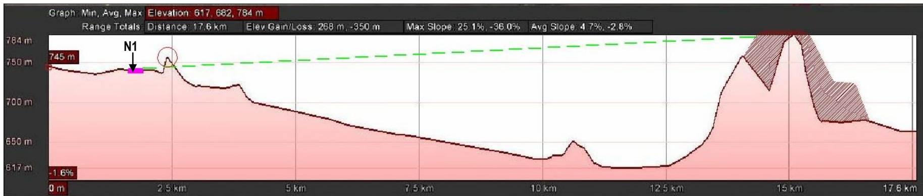
Figure 17: Cross Section F conceptually illustrating the proposed waste dump (hatched area) in relation to surrounding topography and potential receptor sites.
