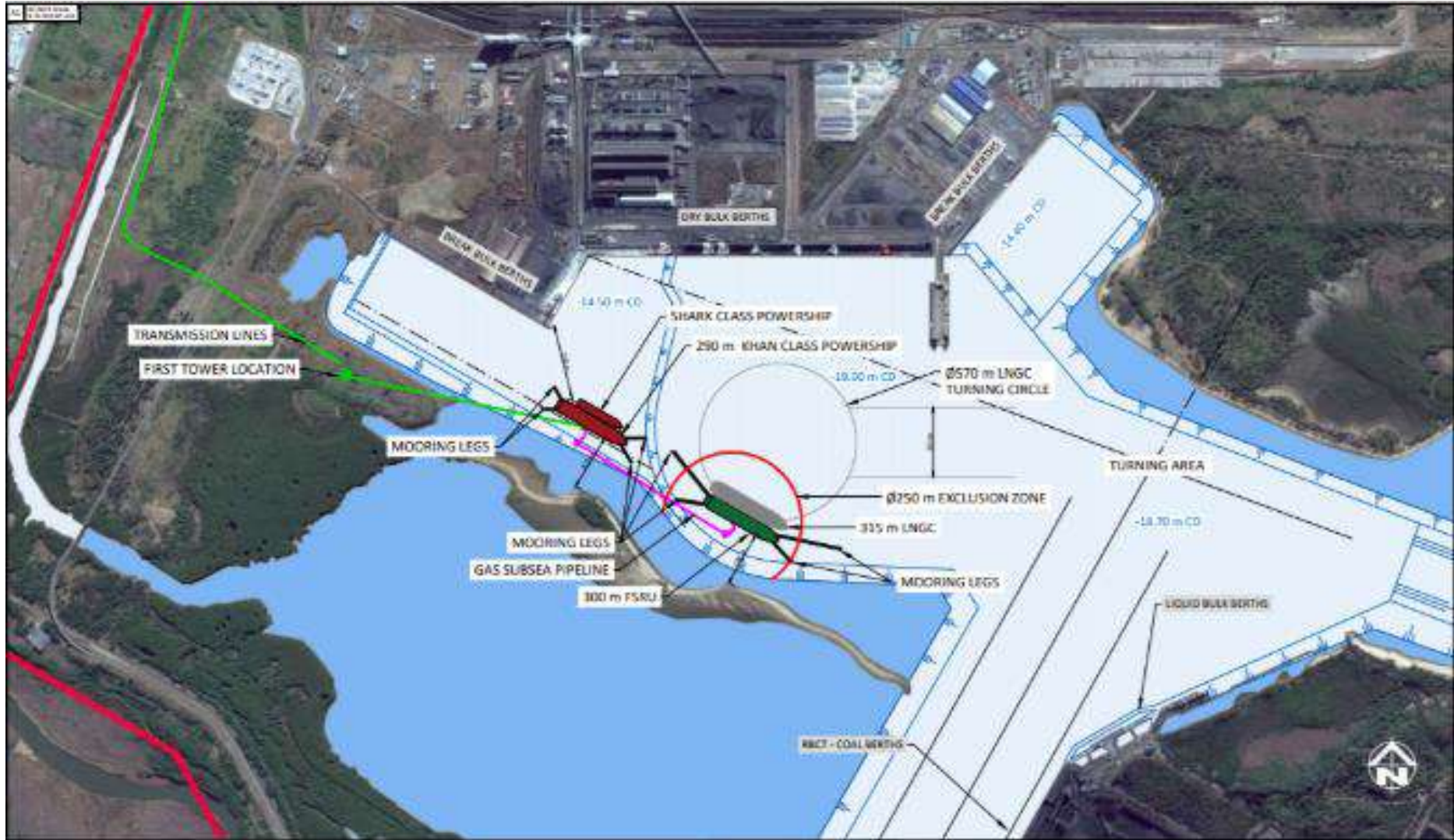
Figure 3-2: Alternative 2: Powerships and FSRU position within the port – further from transmission tower.
