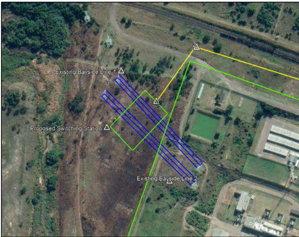
Figure 3-10: Proposed connection to the Eskom line and placement of the switching station.
