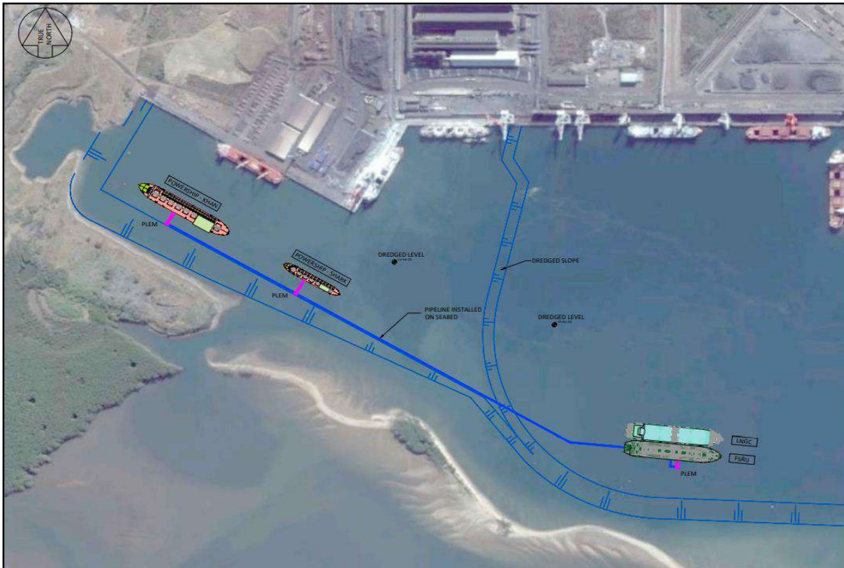
Figure 9-1: Preferred Alternative for the Powerships and FSRU position within the port – closer to transmission tower.
