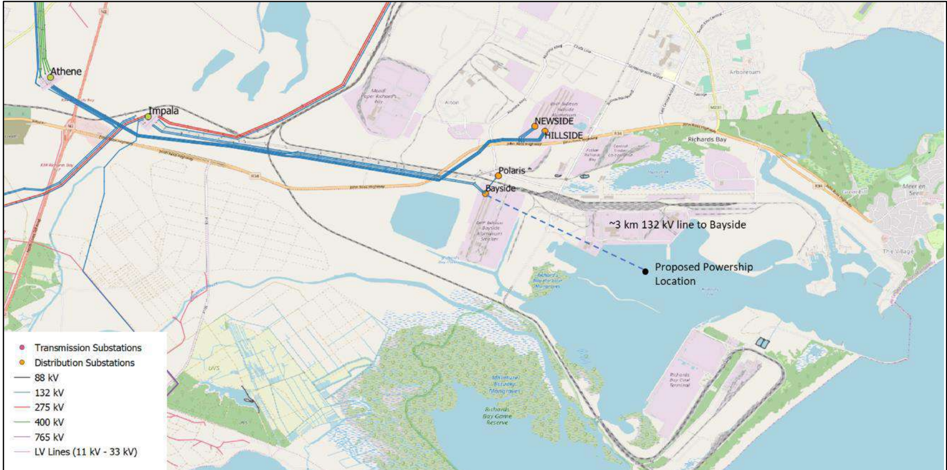
Figure 3-6: 132kV connection near the Bayside Substation in relation to the location of the proposed Powership.
