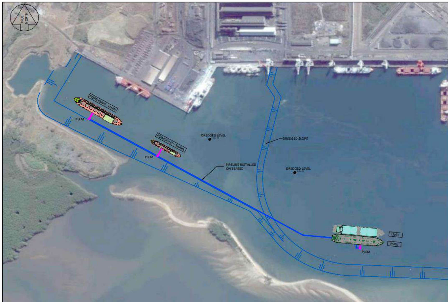
Figure 3-1: Alternative 1 – Preferred: Powerships and FSRU position within the port – closer to transmission tower.
