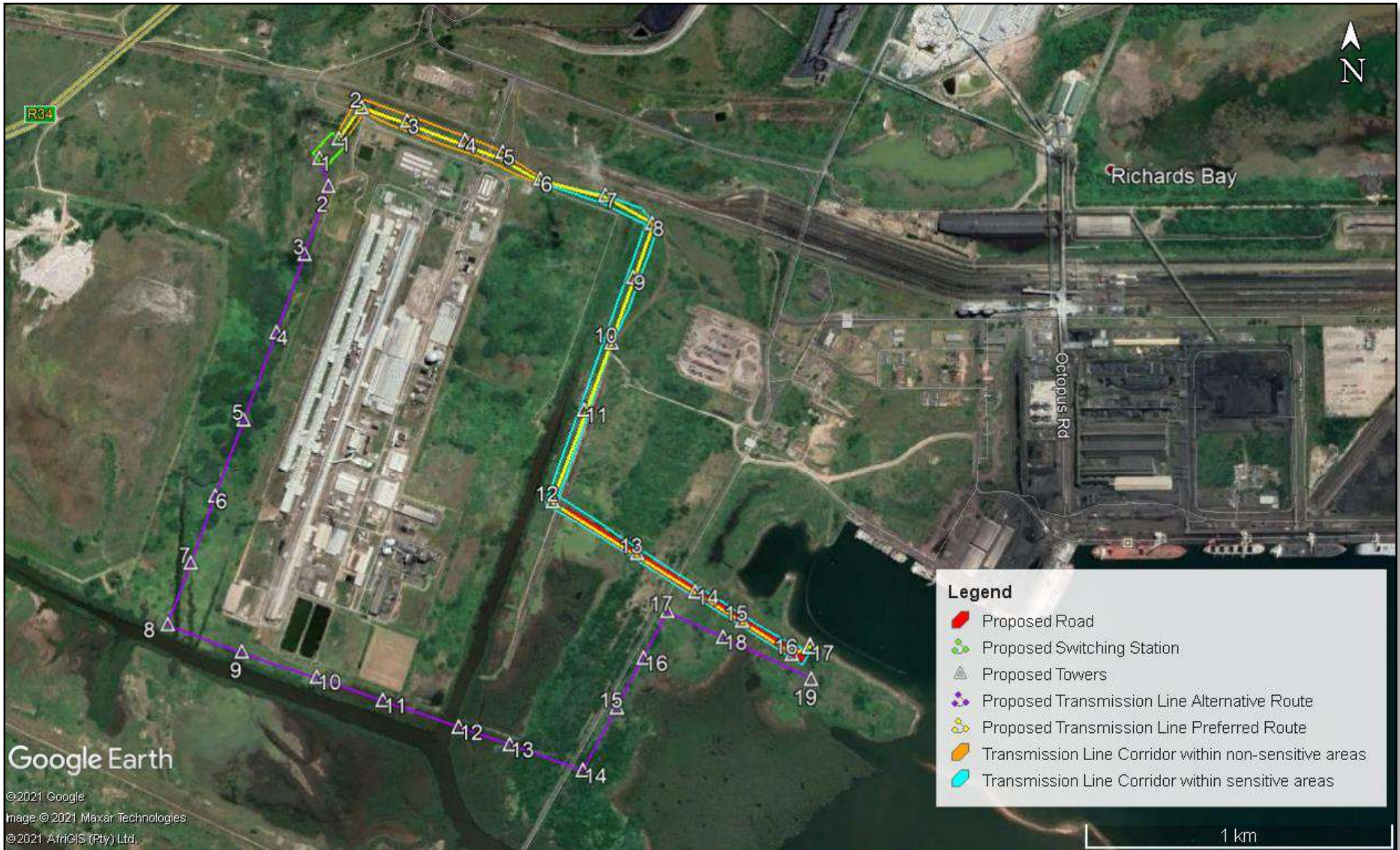
Figure 3-7: Transmission line route alternatives from the Powerships to the proposed switching station – Alternative 1 route and corridor (yellow) and Alternative 2 (purple).
