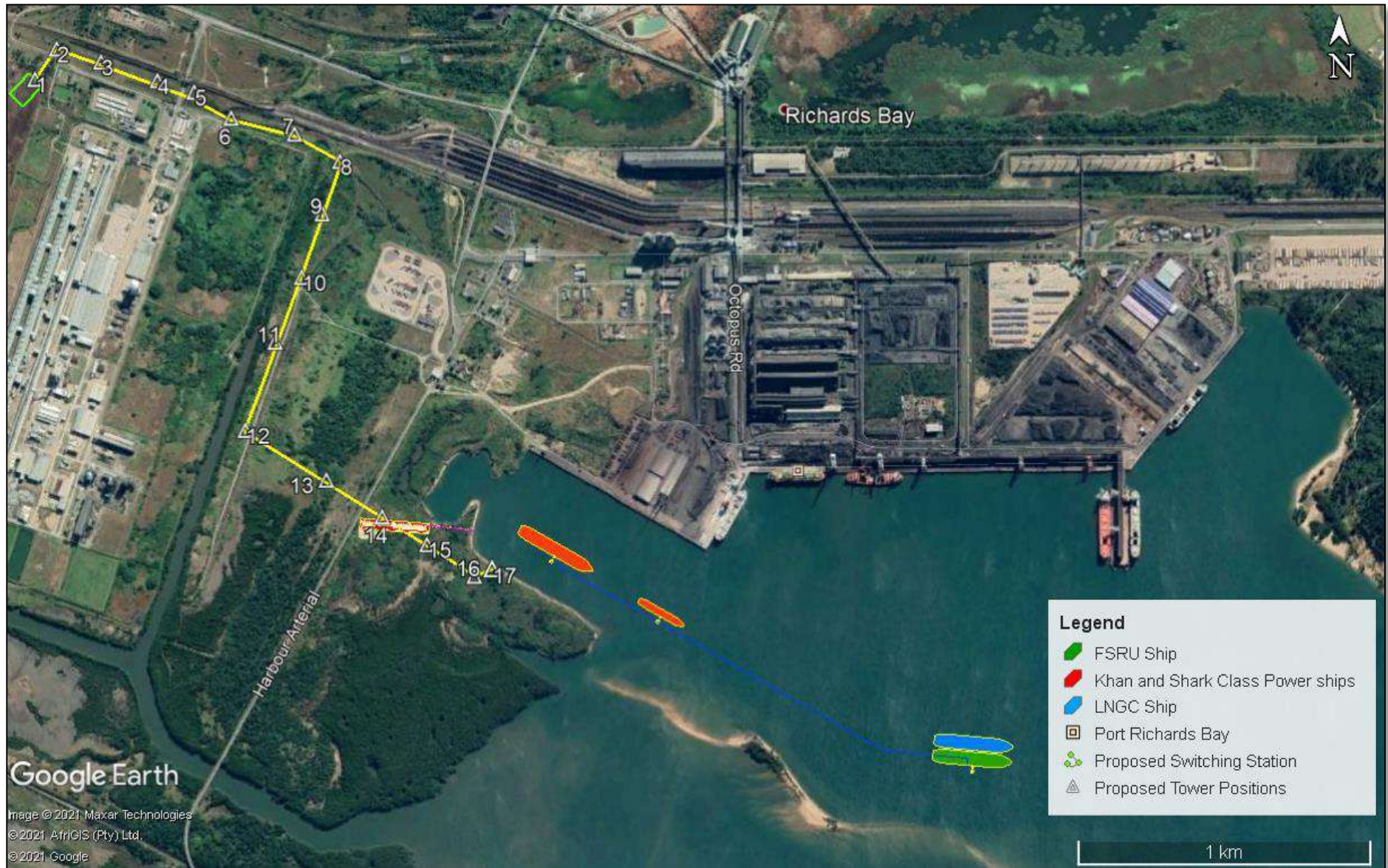
Figure 2-6: Google image showing the proposed Gas to Power Project (preferred alternatives) - Port of Richards Bay.
