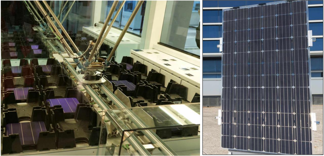
Figure 3-1: PV cells (left) and panel (right)
