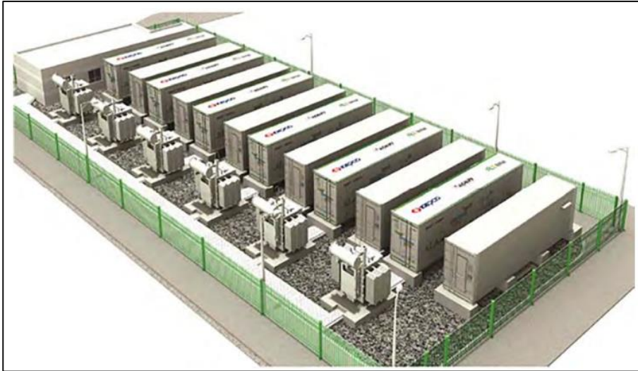
Figure 17: Typical illustration of a battery energy storage system technology 11
