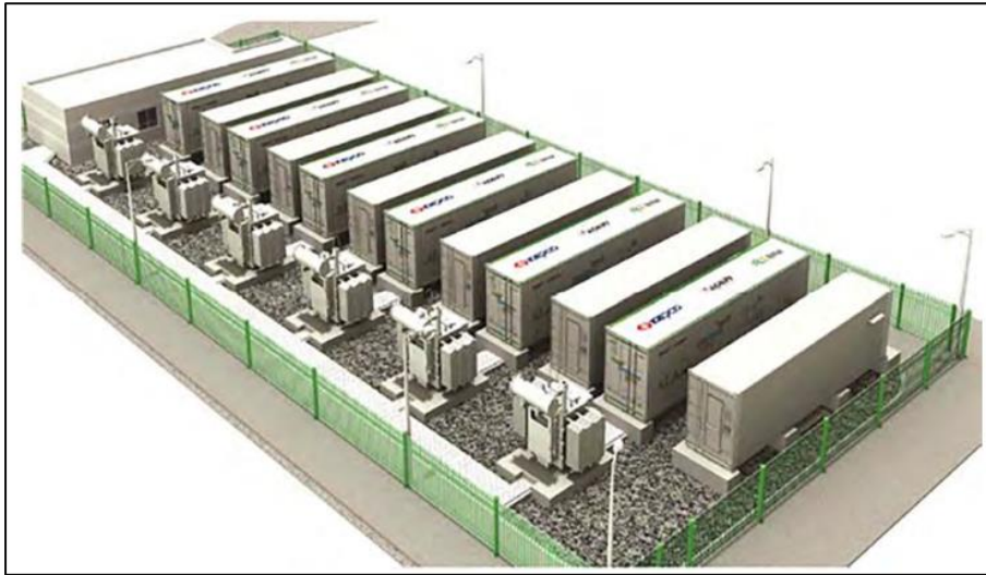
FIGURE 17: TYPICAL ILLUSTRATION OF A BATTERY ENERGY STORAGE SYSTEM TECHNOLOGY 10
