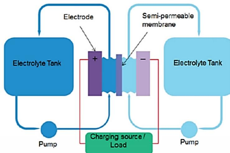
**Figure 2.7: Schematic diagram of a typical Redox Flow Battery (Source: Parsons, 2017<sup>4</sup>)**
