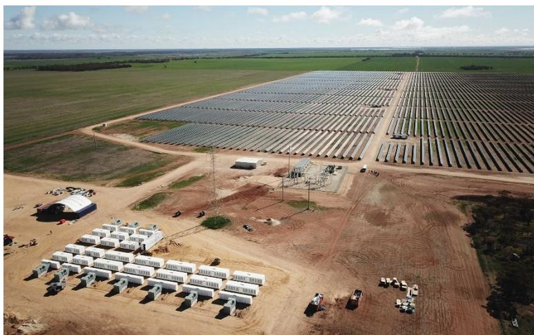
**Figure 2.6. Example of PV Technology with Lithium Ion BESS (ARENAWIRE, 2018<sup>3</sup>)**
