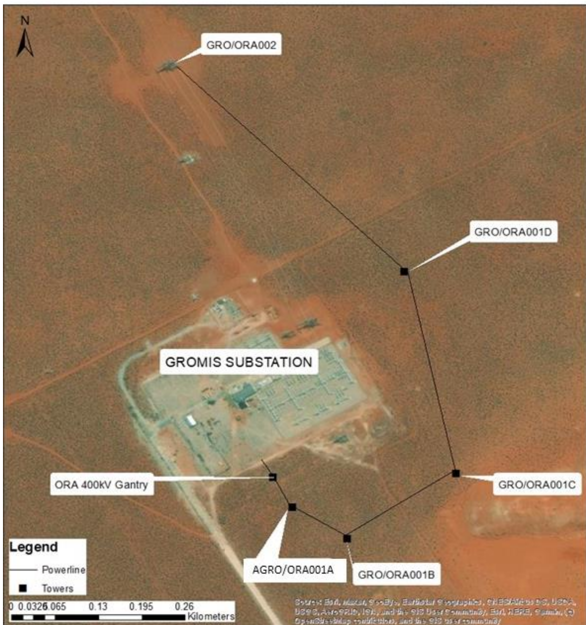
Figure 8: Infrastructure map showing the deviation from the existing tower GRO/ORA002 to GRO/ORA001D, GRO/ORA001C, GRO/ORA001B, GRO/ORA001A and on to the terminal tower.
