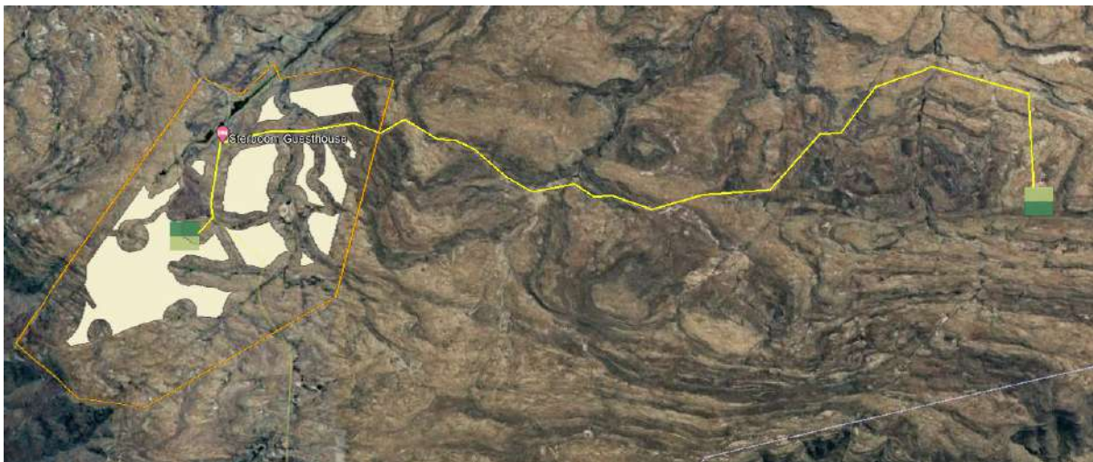
Figure 1.1: Buildable area of the proposed Sutherland 2 WEF (white shaded areas – as surveyed during the pre-construction walkthrough) with the proposed routing for the authorised 132kV powerline (yellow) between the substations.
