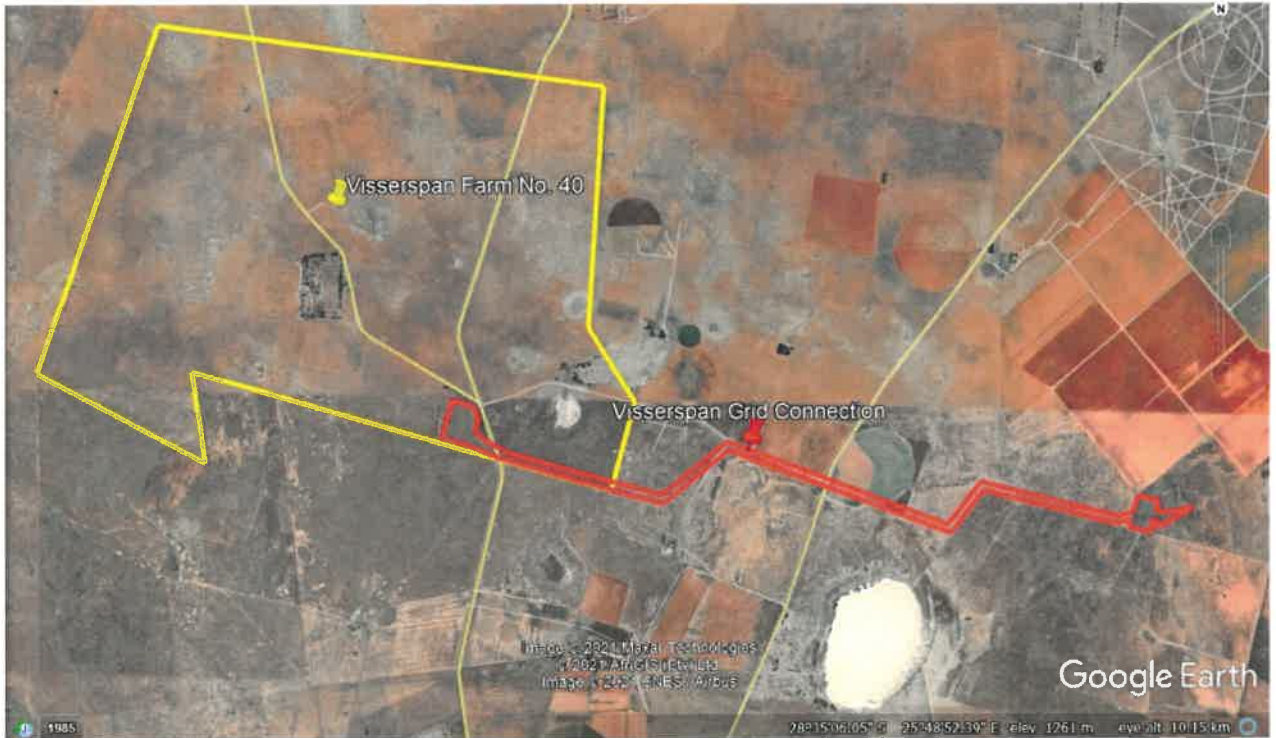
Figure 3: Indication of property (yellow pin and outline) where solar power will be generated utilising four 75MW to 100MW PV facilities i.e. total power to be produced on Visserspan Farm will be not more than 400 MW. Evacuated power will emanate from Visserspan Farm No. 40, Tokologo Local Municipality, Lejweleputswa District Municipality, Boshoff Registration Division, Free State Province and run towards the east (linear route indicated in red).
