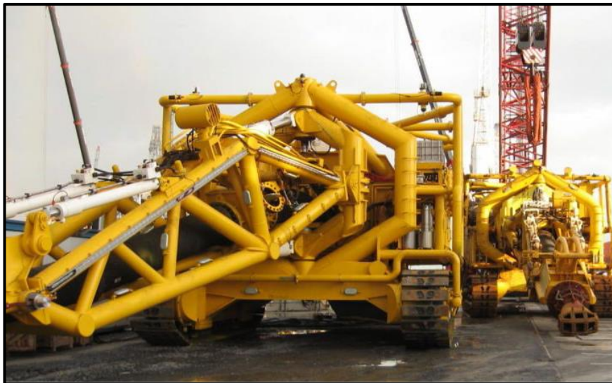
Figure 10: Example of a track-mounted sub-sea crawler
