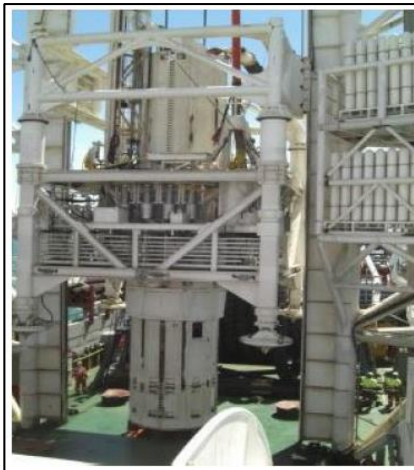
Figure 8: Example of the 2.5 m diameter drill bit within the drill frame structure
