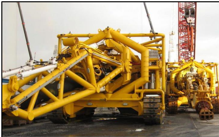
Figure 21: Example of a track-mounted sub-sea crawler
