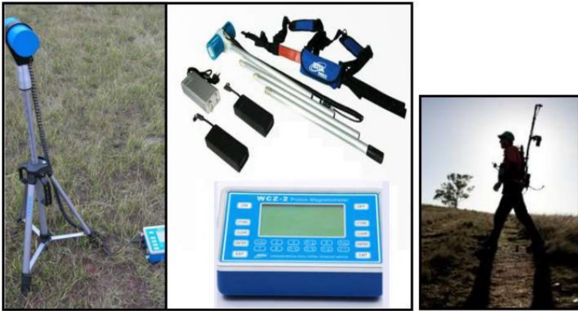
Figure 4: Typical Proton Magnetometer (Source: www.geophysical-equipments.com)
