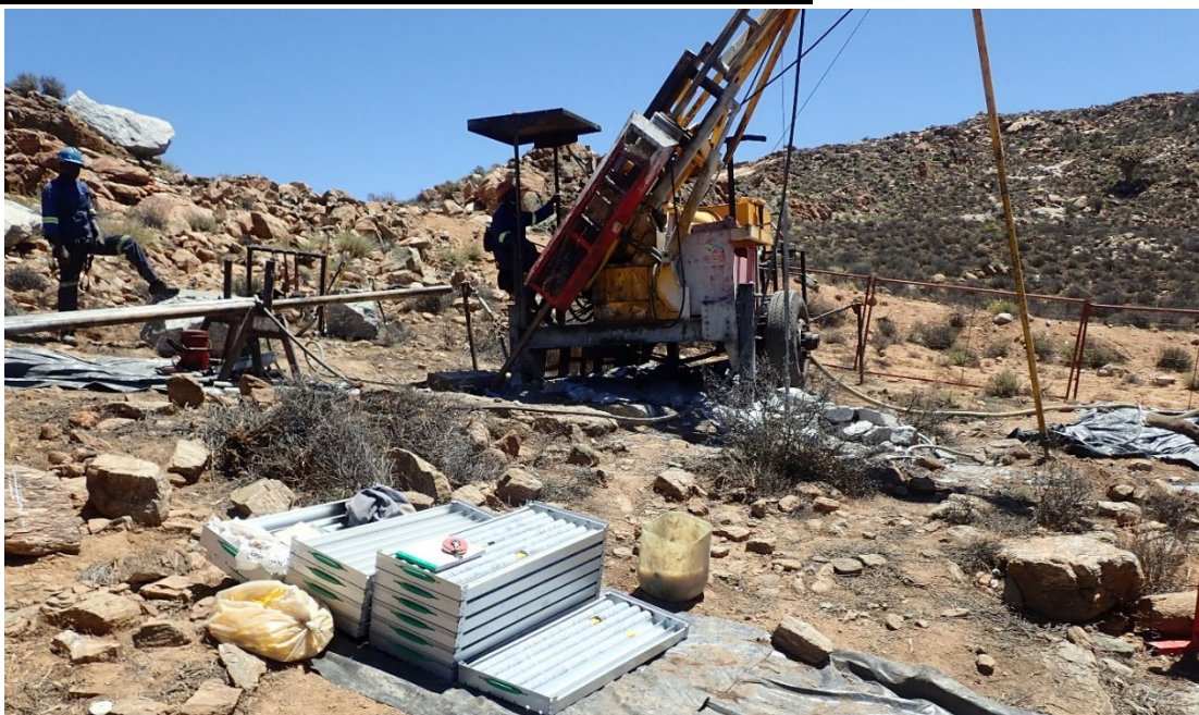
Figure 3b Typical configuration of a diamond drill rig
