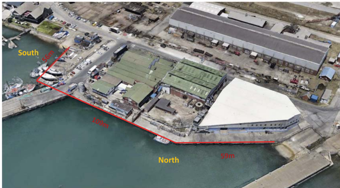
Figure 4-1: Old Tug Jetty Sheetpile layout
