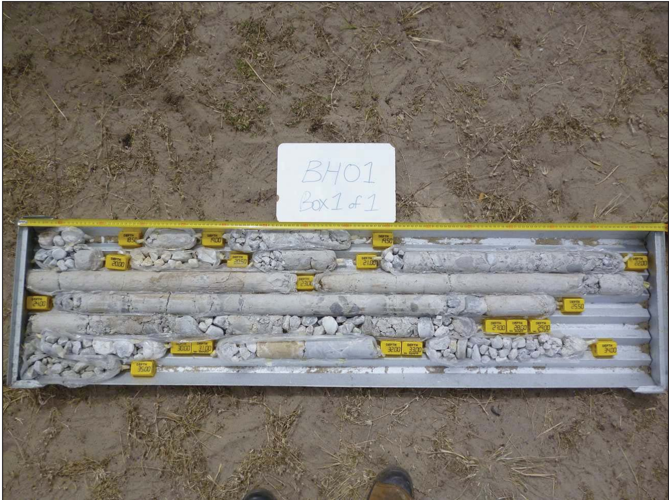
PLATE 1: Borehole core for BH01 from depth 18.40 m – 35.00 m.
