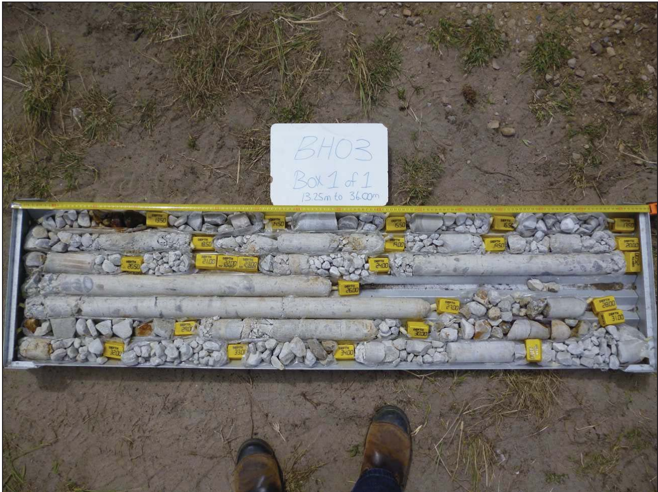
PLATE 3: Borehole core for BH03 from depth 13.25 m – 36.00 m.
