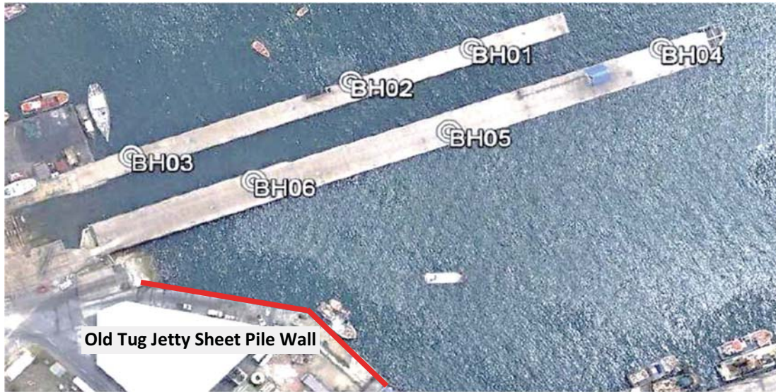
Figure 2-3: Lead-in jetty borehole locations
