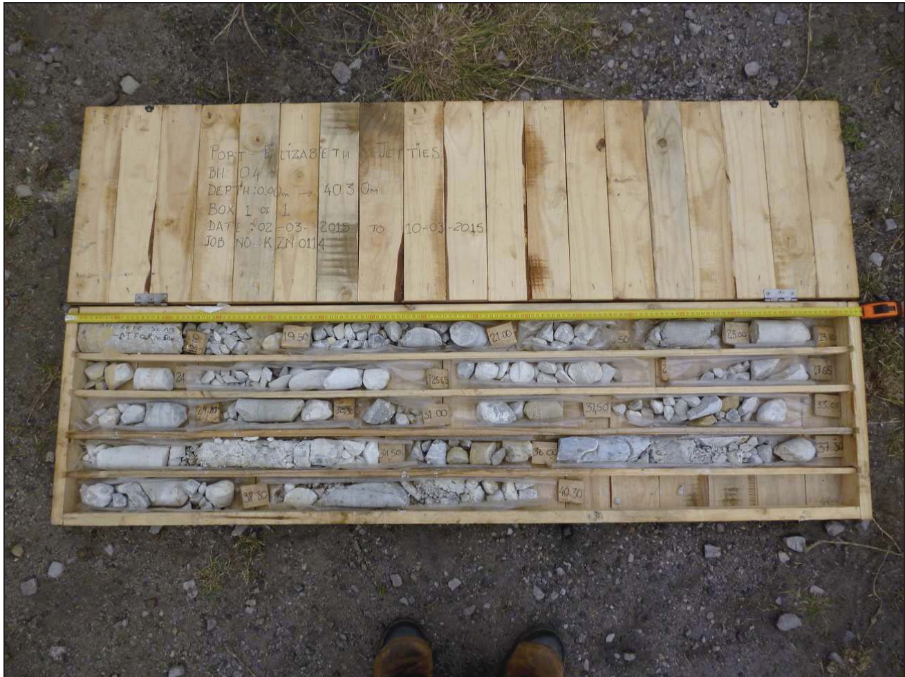
PLATE 4: Borehole core for BH04 from depth 18.00 m – 40.30 m.
