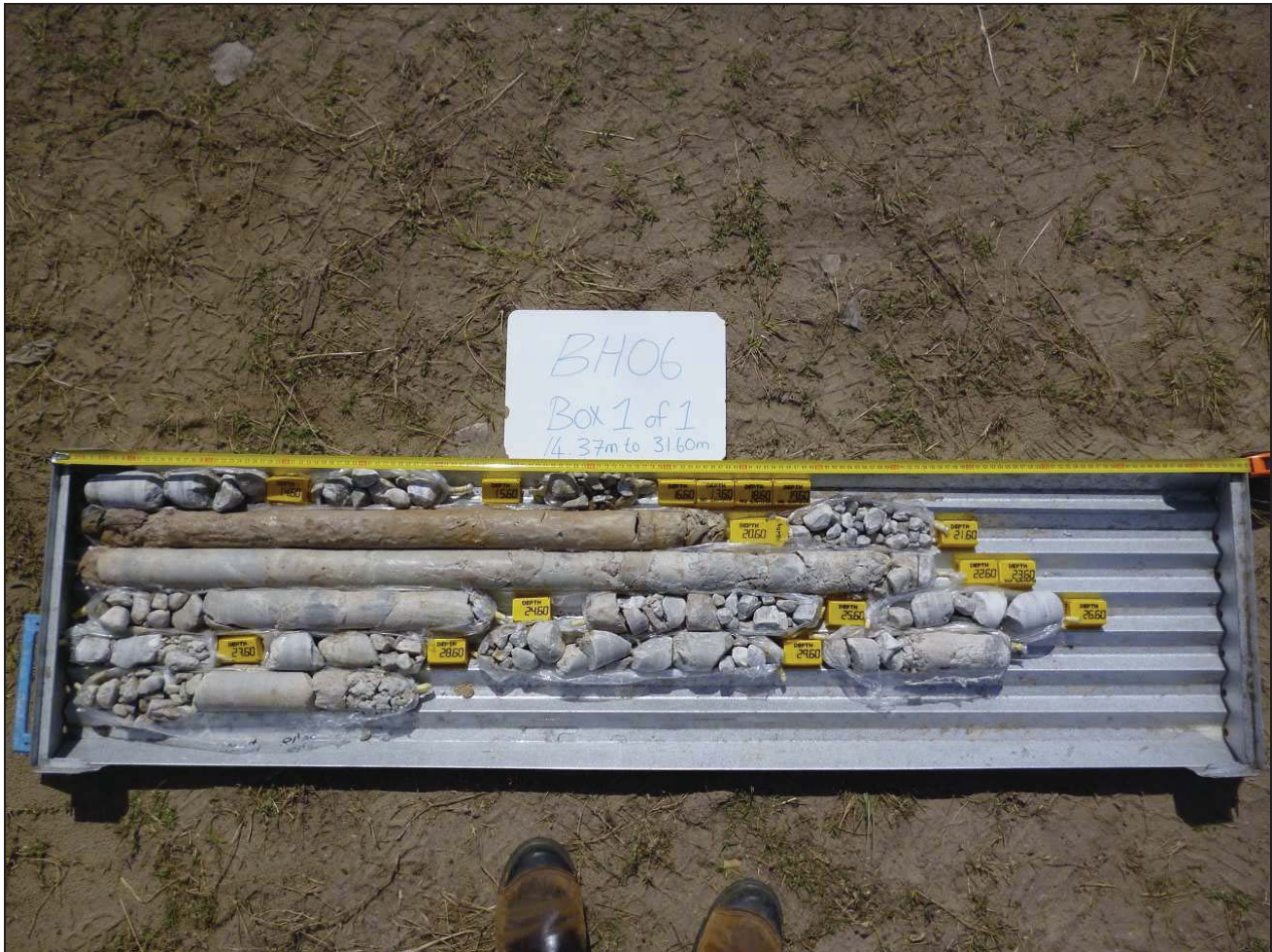
PLATE 6: Borehole core for BH06 from depth 14.37 m – 31.60 m.
