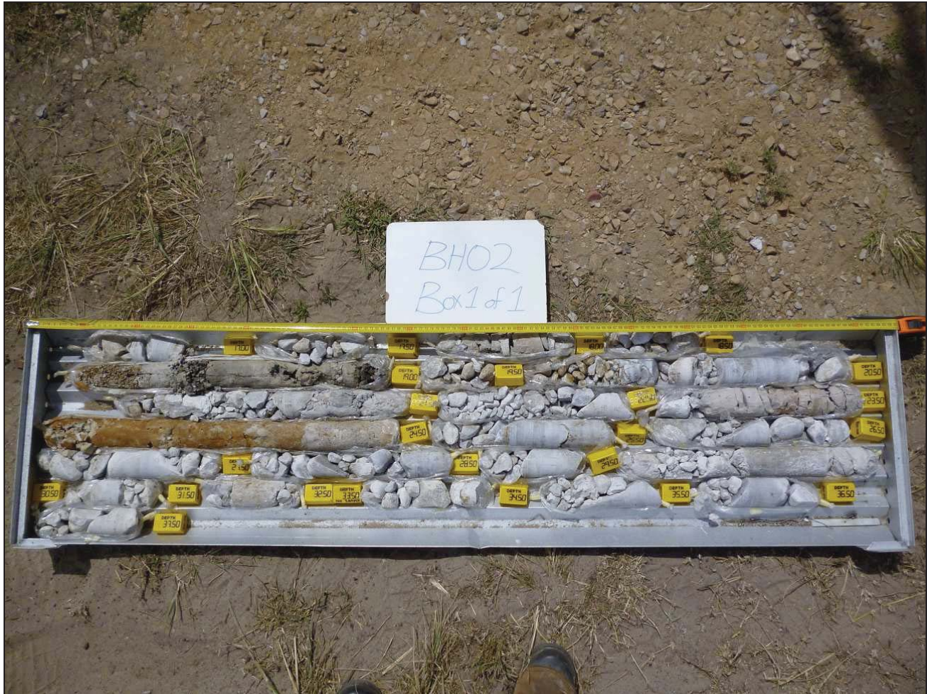
PLATE 2: Borehole core for BH02 from depth 16.80 m – 37.50 m.
