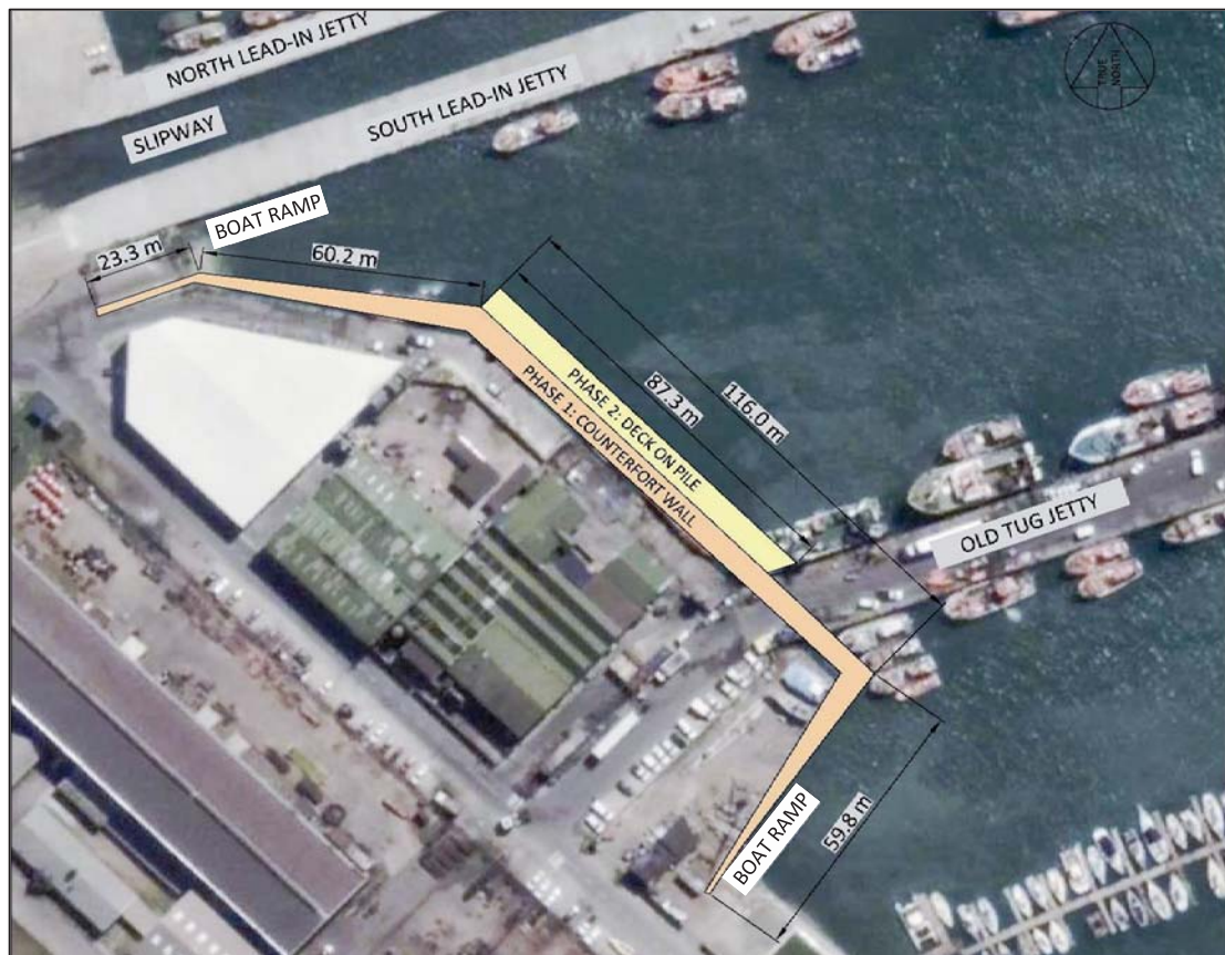
Figure 2-1: Phase construction of preferred solution
