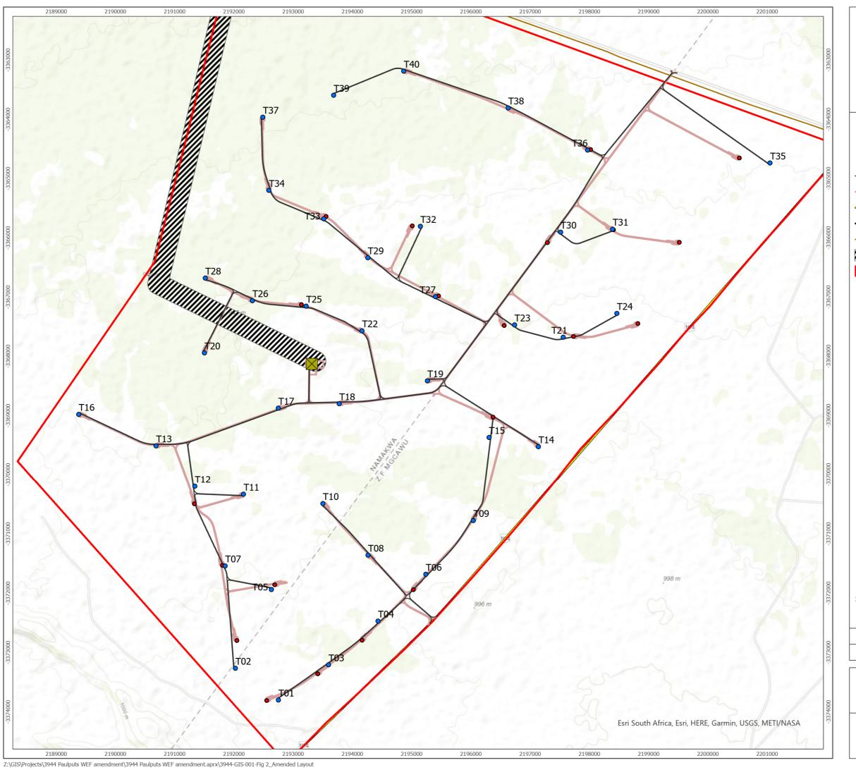
**\$**ARCUS Substation Compound Option A Amended WTG Layout Approved Paulputs Turbine Placement - Amended Internal Roads Roads, Hardstands and Substations N14 Highway ---- R358 Unclassified Road Approved Paulputs WEF Corridor Paulputs North WEF Site 1:45 000 Scale @ A3 1,7 km Ref: 3944-GIS-002 Produced By: ABL Date: 2021/07/22 Checked By: MB
