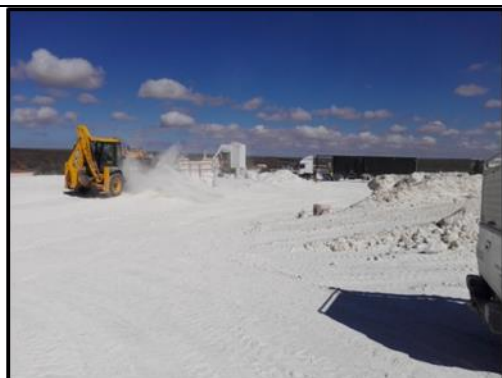
Photograph 2: View of the Backhoe Actor that runs back and forth to crush the kaolin into a powder form.
