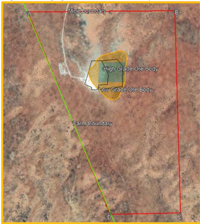
Diagram 3: Mining Right Area Mineral Resource Map for Identified Orebody showing grades of ore body
