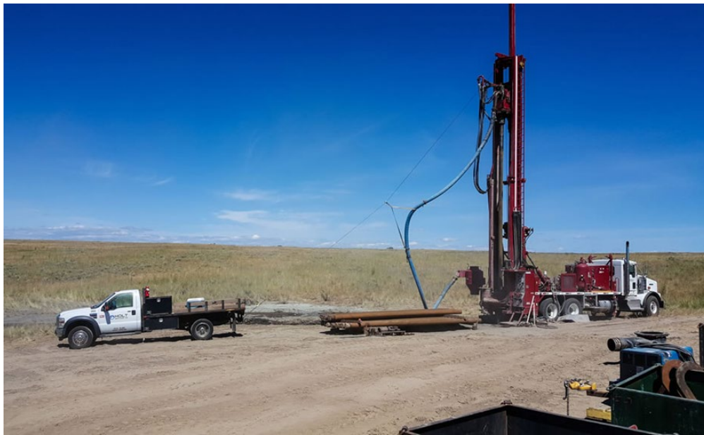
Figure 4 Typical configuration of a diamond drill rig
