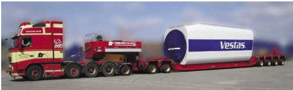
*Figure 4-1:Transporting the Nacelle (Dvorak, 2010)*
