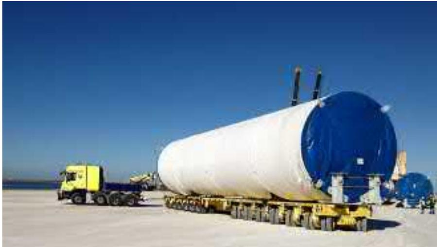
*Figure 4-3:Transporting the Tower Sections (Montiea, 2014)*
