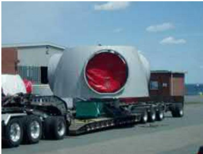
*Figure 4-4:Transporting the rotor hub (Richardstransport, n.d.)*
