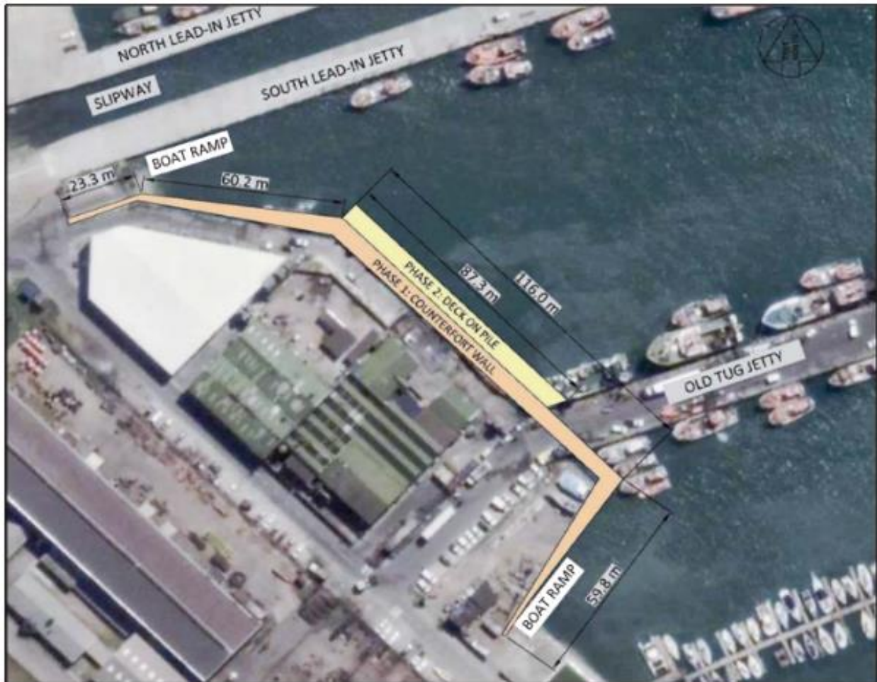
Figure 4: Phase construction of preferred solution
