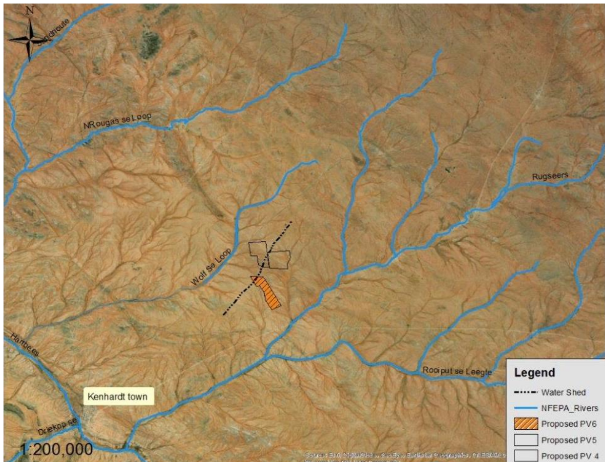
Figure 5: Map indicating drainage lines associated with Kenhardt PV6, indicating that the site lies within the catchment of the Rugseersrivier system.
