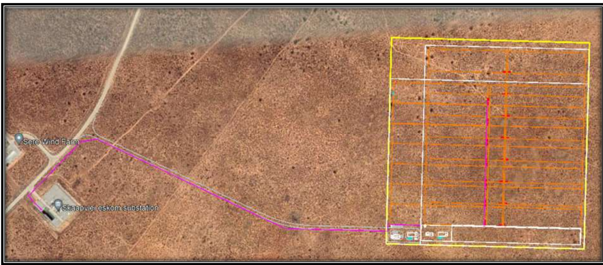
Figure 3: Alternative 1 - Fixed and Tracking layouts within the Assessment Site Boundary (yellow) showing cable and access road routes.
