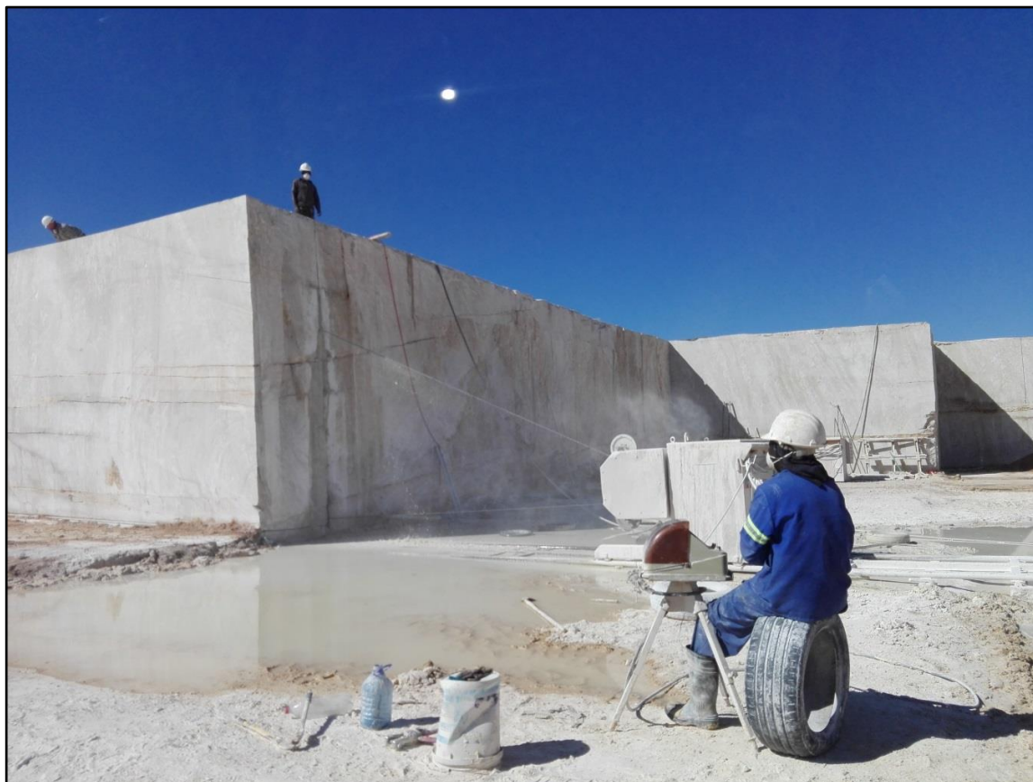
Photograph 2: Diamond-impregnated wire saw in action at Yellow Quarry 1.
