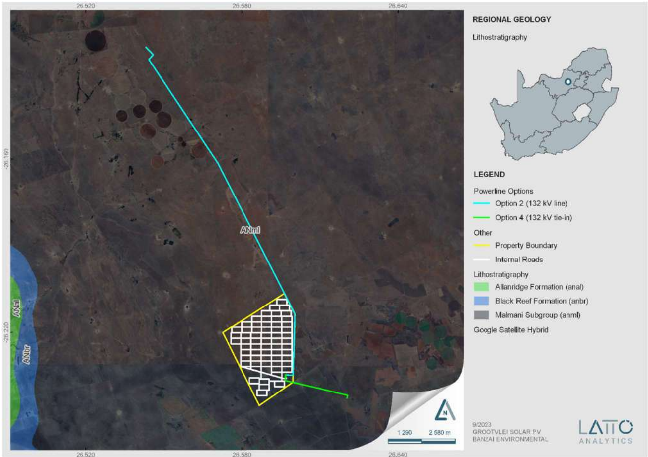
Figure 7: Updated Geology (Council of Geosciences, Pretoria) of the study area indicates that the development is underlain by the Malmani Subgroup (Chuniespoort Group, Transvaal Supergroup).
