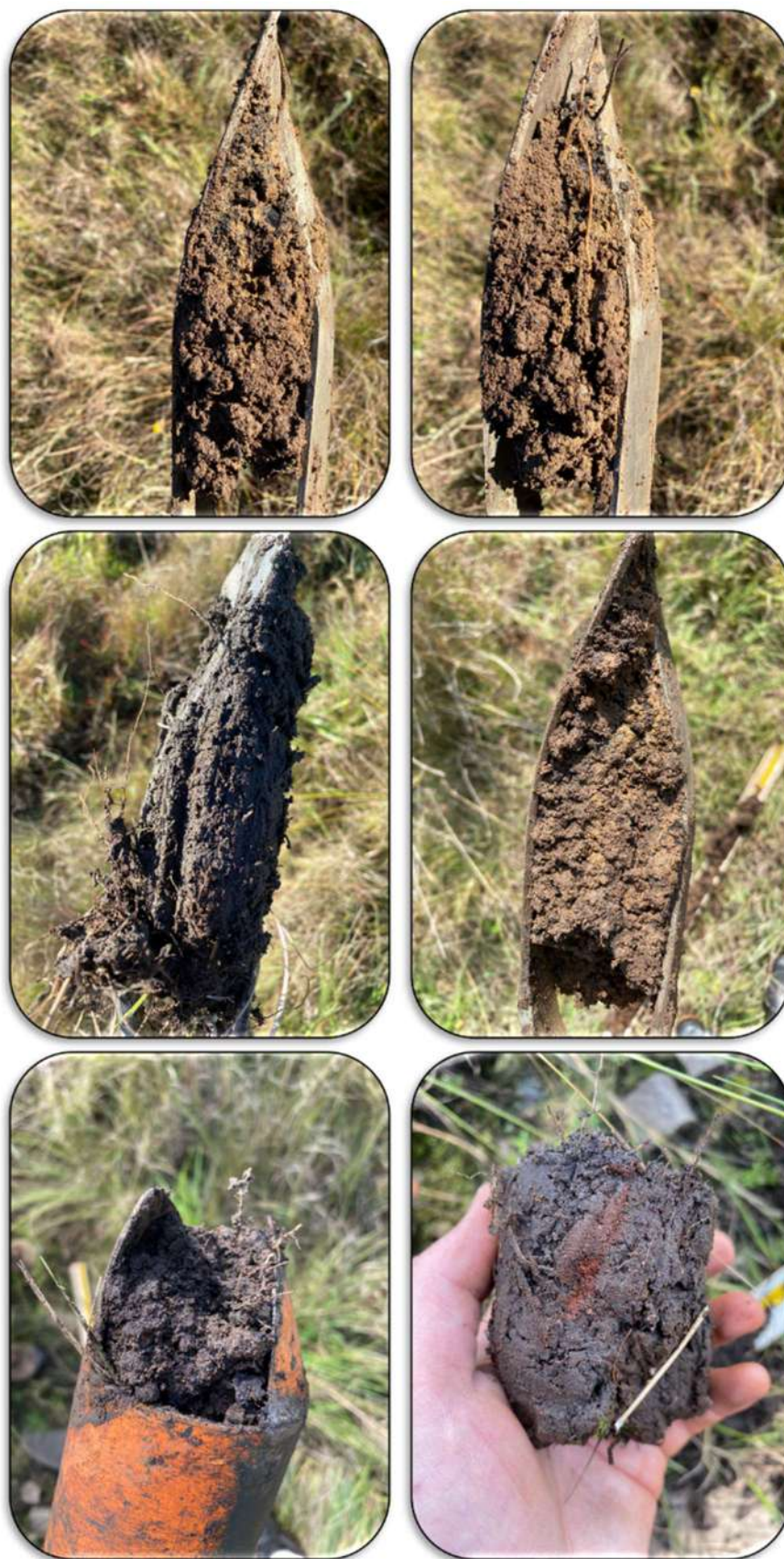
Figure 30: Soil samples collected showing the strong clay content in soil as well red-yellow mottling. Soil types is mostly comprised of Glenrosa soils
