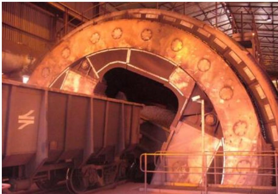
Figure 5-1: Typical enclosed rotary tippler (Transnet, 2012)
