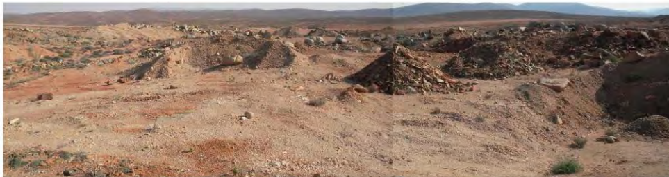
Figure 25: Overburden dumps to be backfilled by means of loading and hauling
