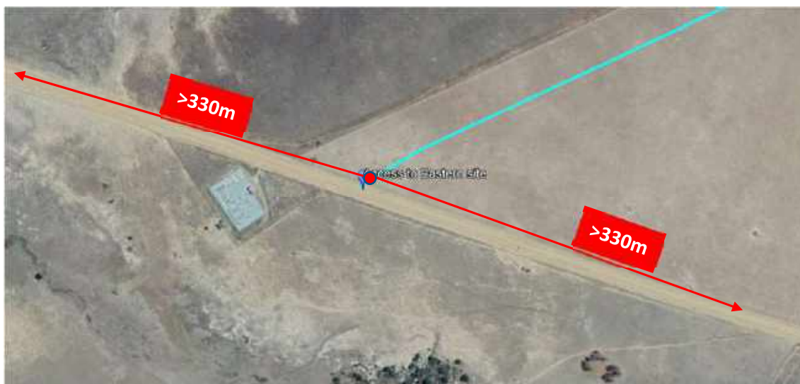
Figure 4-8: Sight distances at Eastern access
