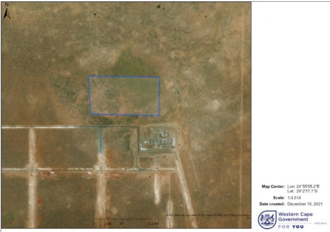
C6: Bing satellite image showing proposed BESS Alternative 1 footprint (blue polygon) within wetland depression.
