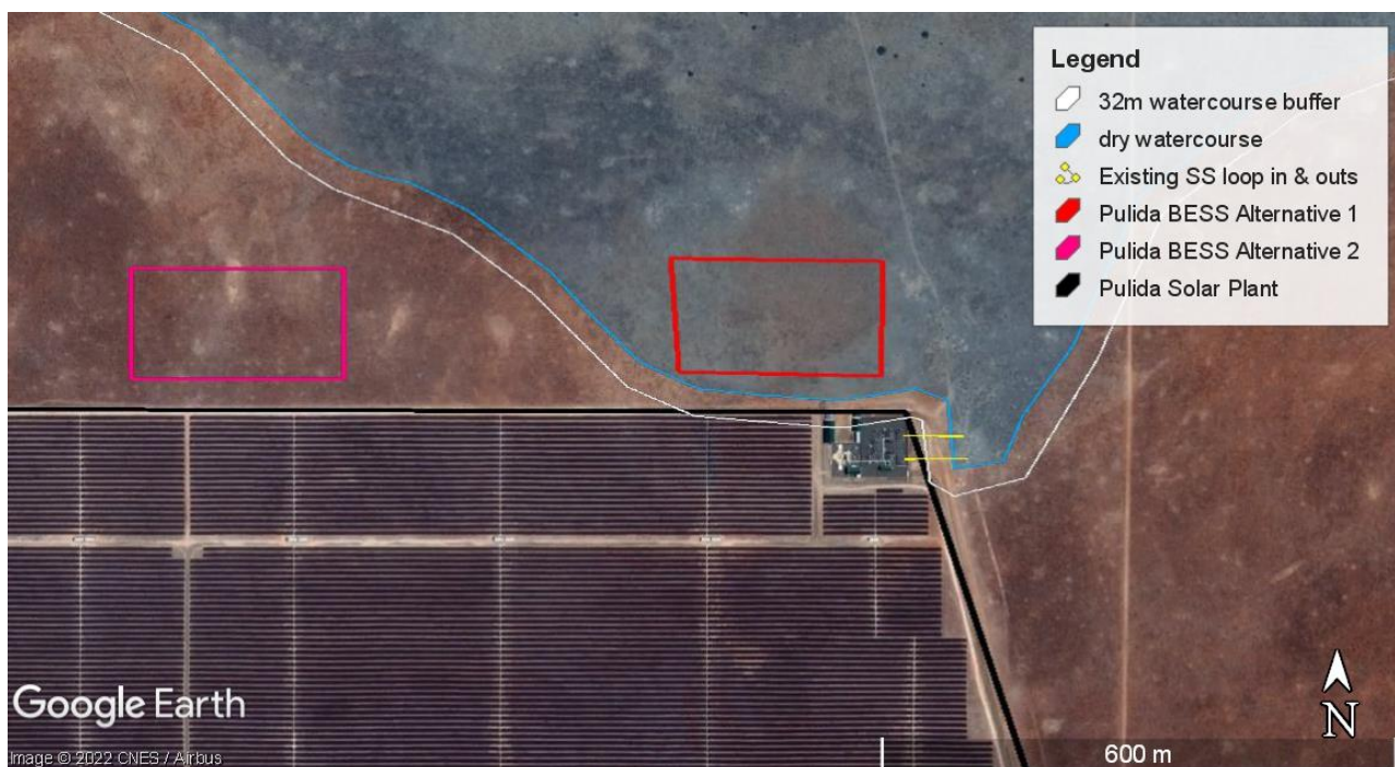
Figure 4-4b: Site map of the watercourse and 32m buffer in relation to the alternative BESS sites and the existing Pulida Solar Plant (Source: Google Earth).
