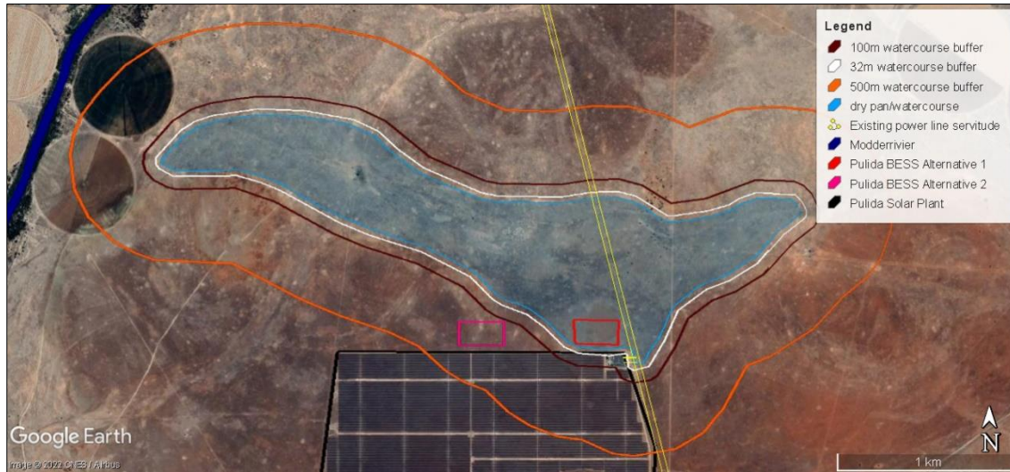
C1: Google map showing depression wetland and the regulated area (32m, 100m and 500m buffer) in relation to BESS Alternatives 1 and 2.
