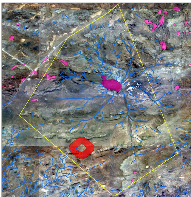
Figure 3 Proximity of NFEPA wetlands (pink) in relation to the preferred BESS site and a 500 m buffer
