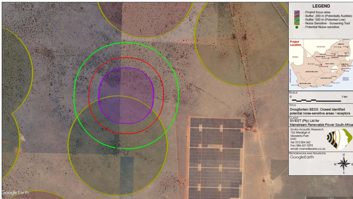
Figure D.1: Screening tool indicating the BESS area falls close to a zone identified to have a potential high noise sensitivity.
