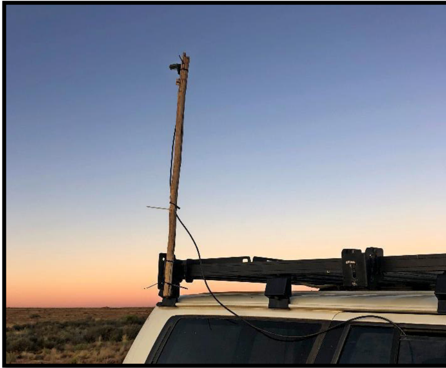
Figure 2-7: Bat detector microphone deployed on a vehicle for use during driven bat transects.
