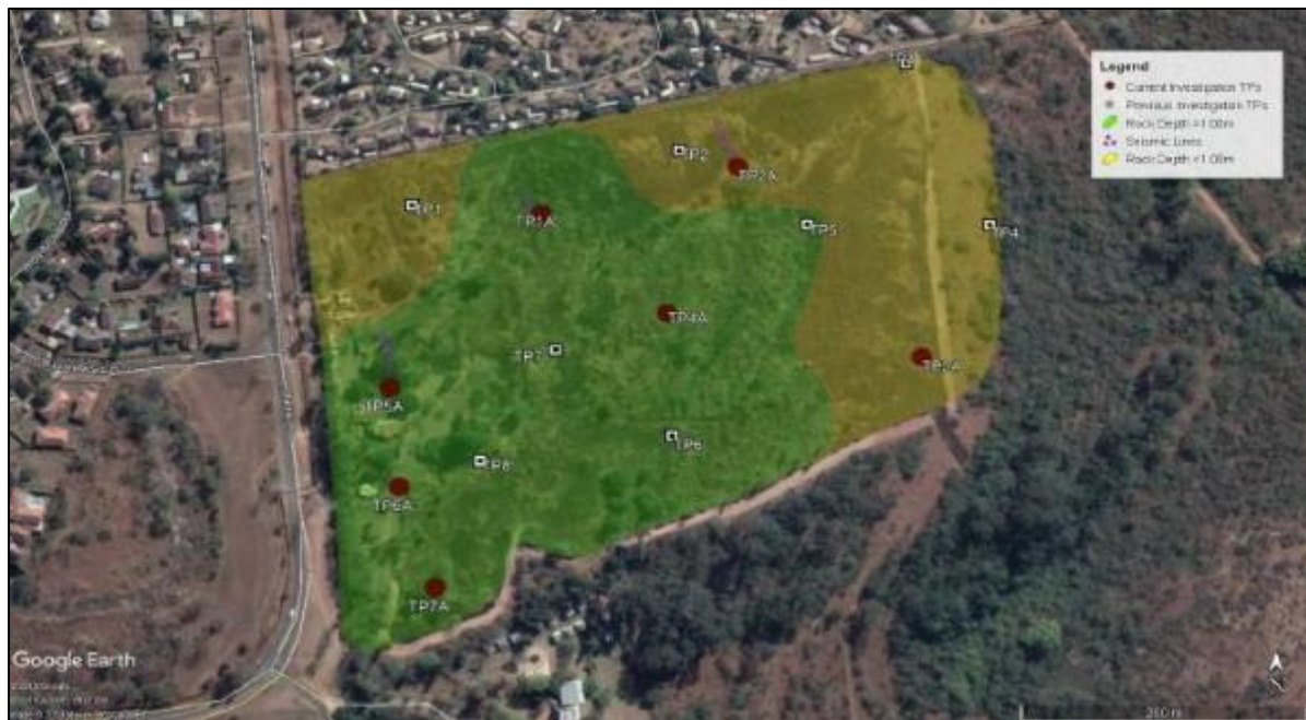
Figure 23: Map showing the location of the investigation test pits and rock depth.
