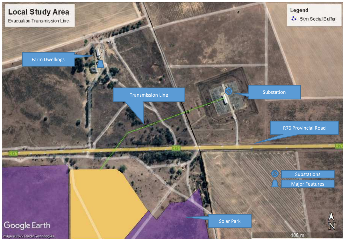
Figure 12: Transmission Line Section of the Proposed Project
