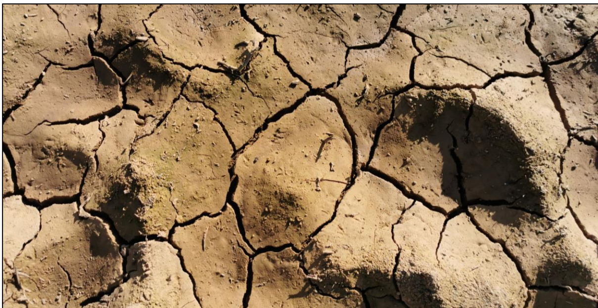
Figure 4-16: Surface silt deposits which occur over an orthic sandy horizon and bedrock indicative of a Clovelly soil form typical in the depression systems (July 2022)
