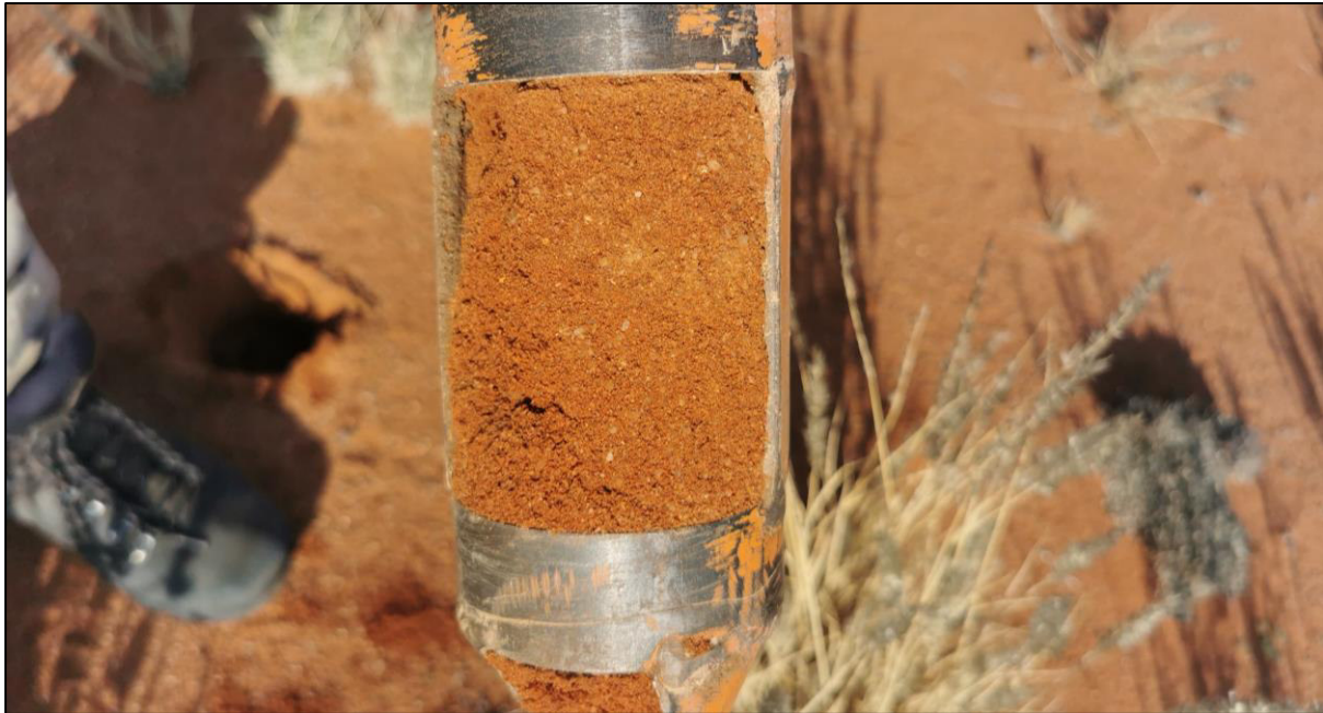
Figure 4-15: Soil types observed in non-perennial washes showing orthic horizons typical in the Clovelly soil form (July 2022)
