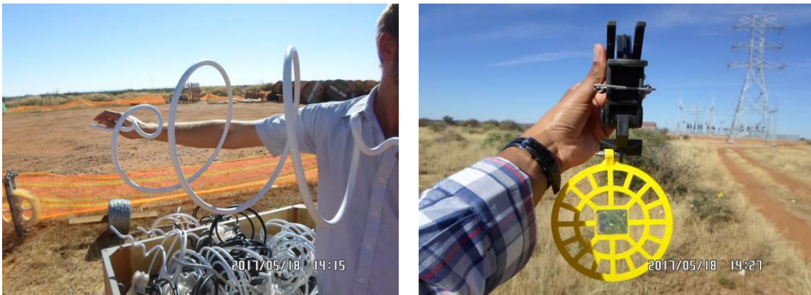
Figure 28: Examples of bird flight diverters to be used on existing power lines: Double loop bird flight diverter (left) and Viper live bird flapper (right).
