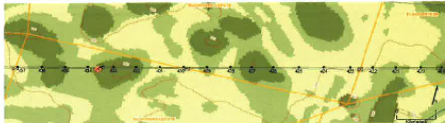
Figure 1: Example of an environmental sensitivity map in the context of a final overhead transmission and distribution profile
