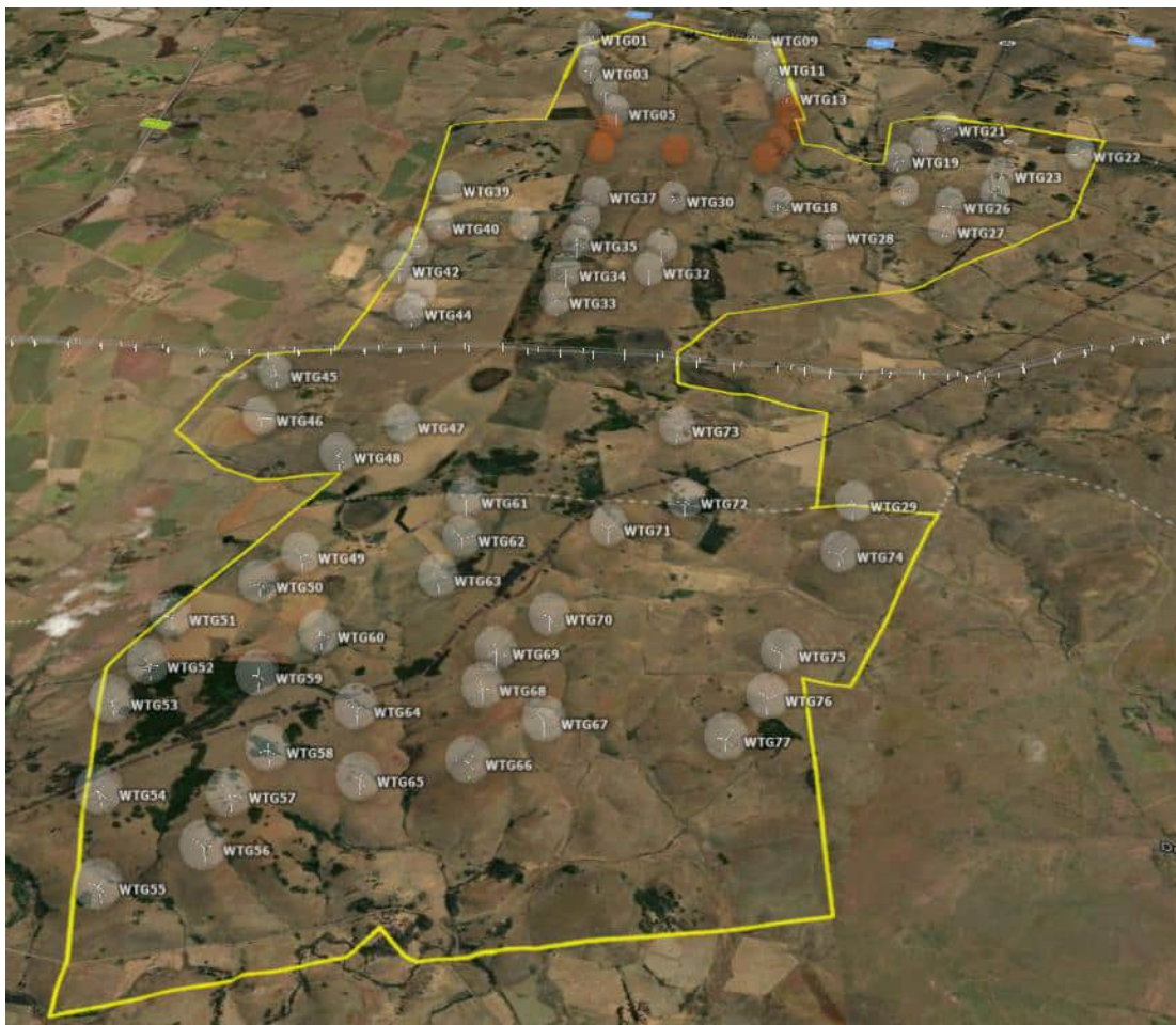
Figure 1 A 3D map drawn to scale in real world units that displays the proposed 70 wind turbines in transparent white, and the 7 sensitive ones that will be removed in reddish-orange. A 100m buffer is created around each wind turbine (based on the length of the rotor blades). The area impacted by the blades is an estimated 418 ha. From the map it is easier to visualise the proposed impact on a landscape with many threatened birds species, with some that are breeding/roosting.
