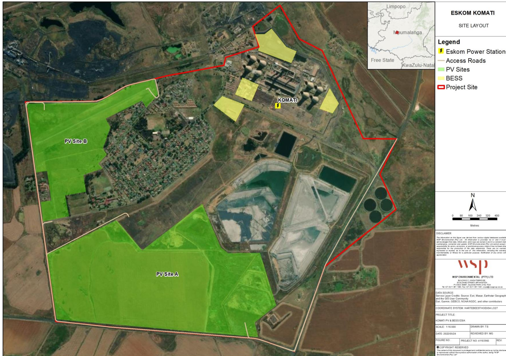
Figure 1: Komati Power Station Solar PV and BESS facilities.
