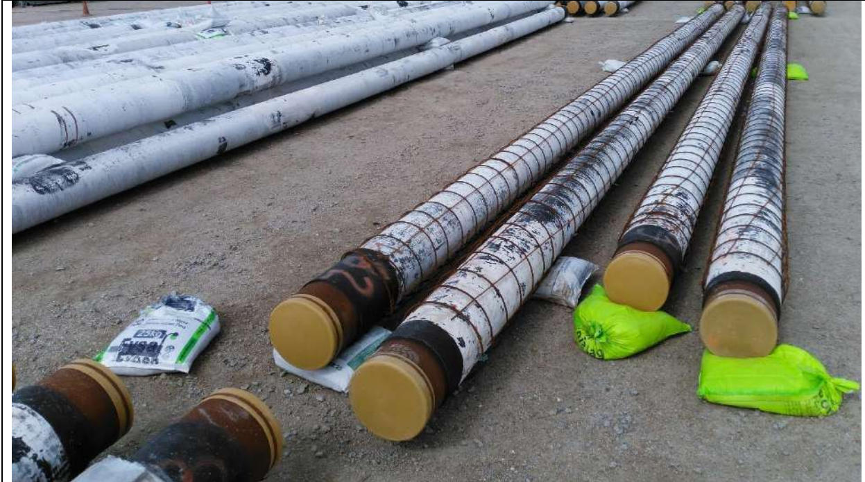
Steel pipes with concrete weight coating in various stages of fabrication pre-installation on the seabed
