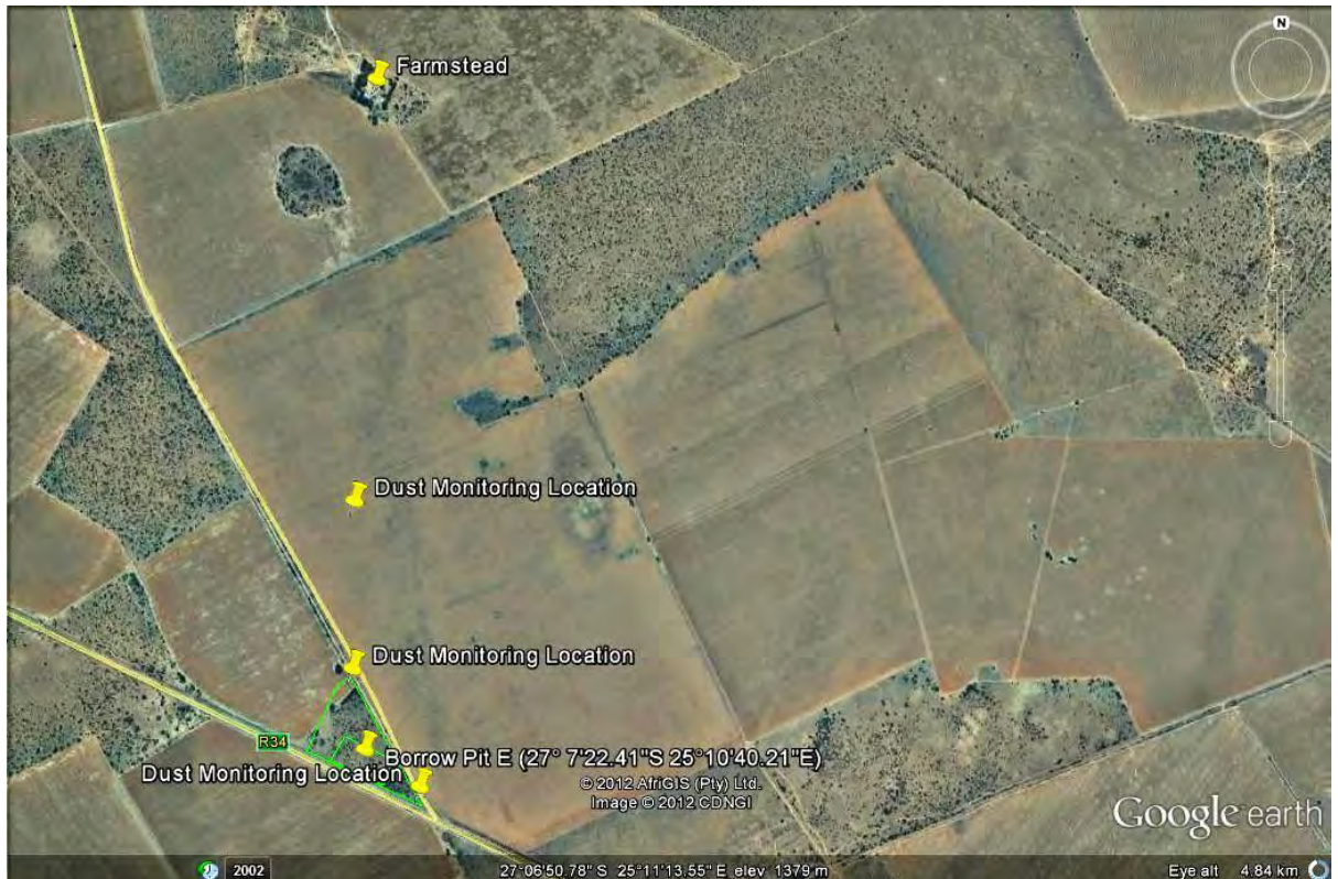
Figure 4 Location of nuisance dust monitoring stations on the NW and SE site perimeter and approximately 0.5 kilometres north of the site and in the direction of the nearest neighbouring property.
