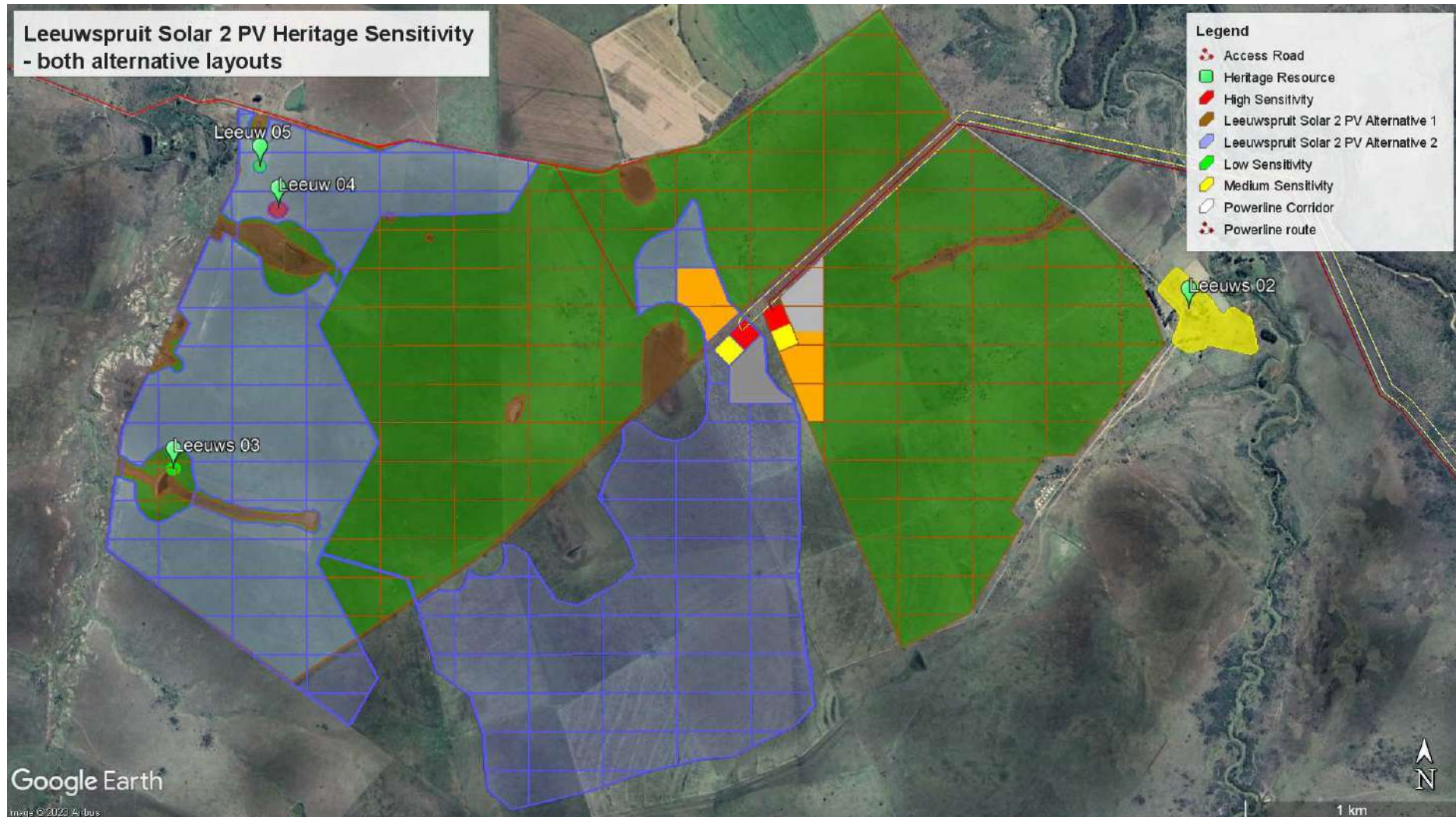
Figure 34: Heritage resources identified during the site survey and overlaid on the project layout, showing Alternative 1 and Alternative 2 layouts
