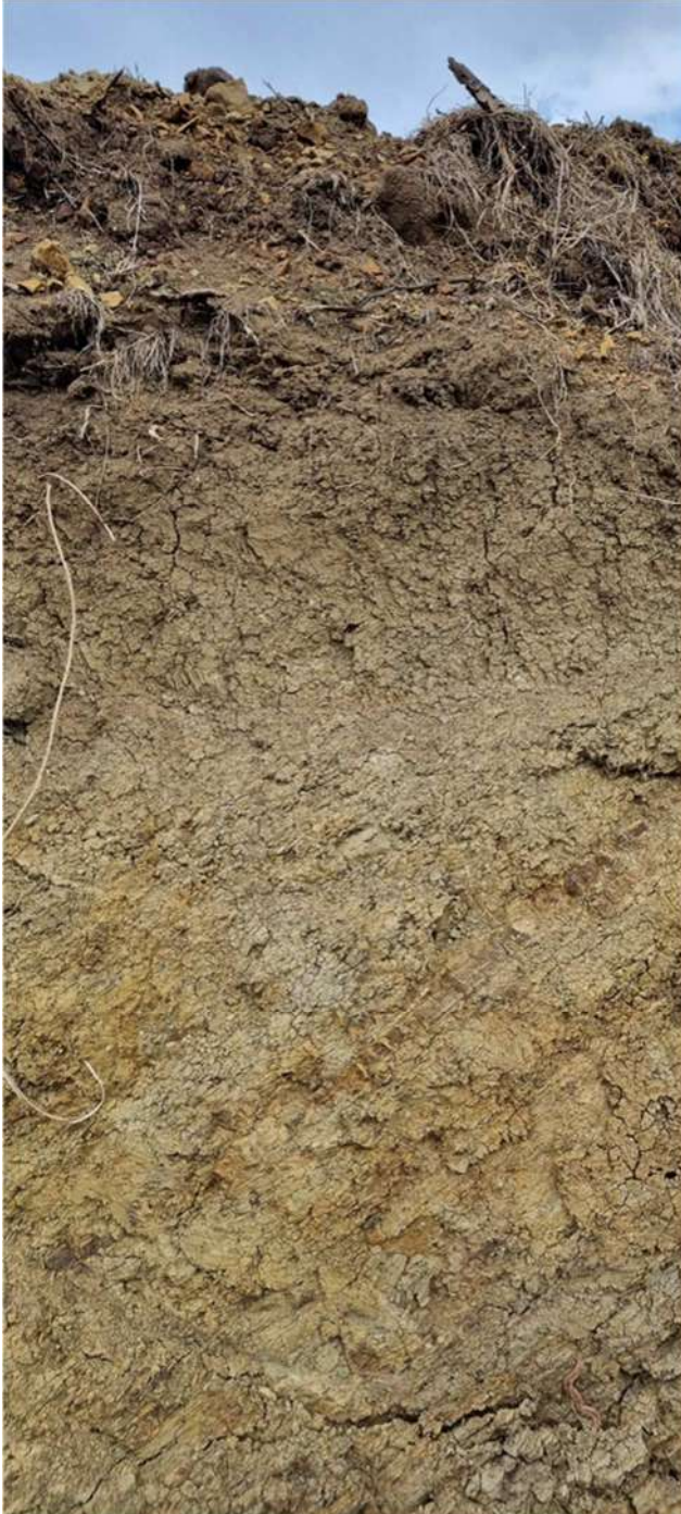
Figure 38: Soil profile in an upper landscape on the farm Mooivlei exhibiting a melanic A horizon on a pedocutanic B horizon with high clay content typical of a Bonheim soil form.
