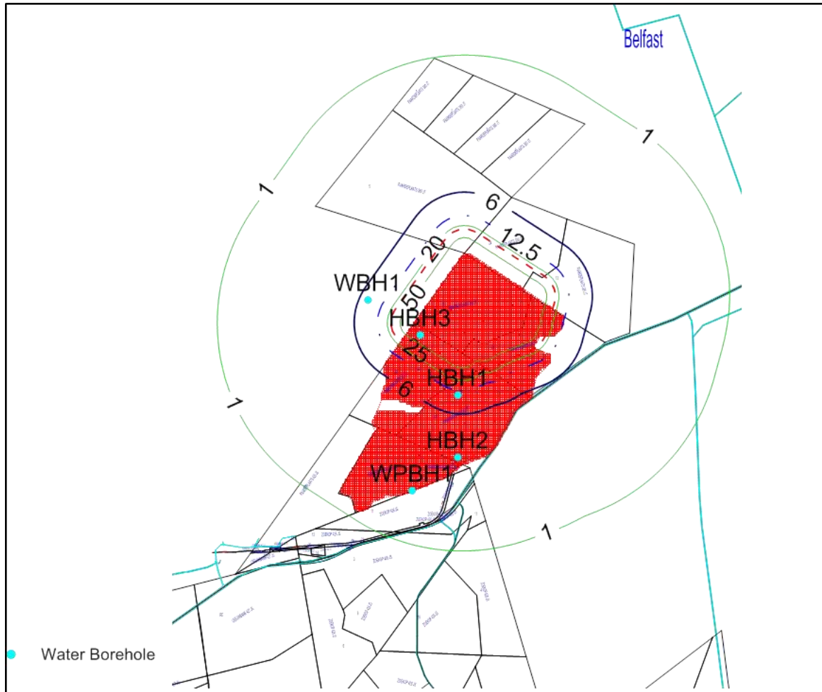
Figure 29: Ground vibration for Portion 30
