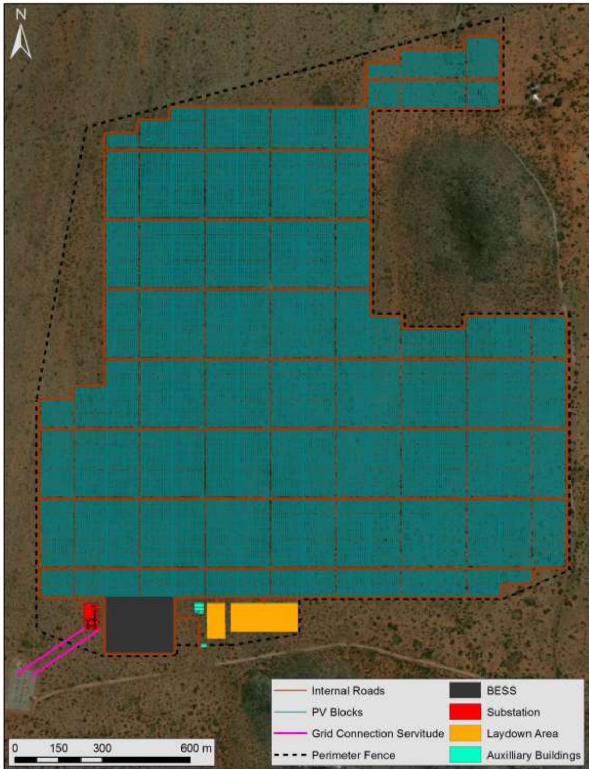
Figure 1. Proposed site layout plan for preferred development option (Postmasburg Solar PV Energy Facility 2)
